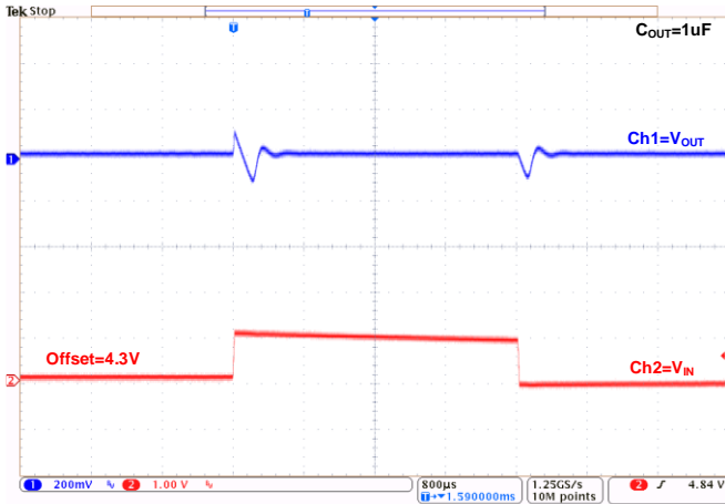
Line Transient at V_{OUT}=3.3V : ( I_{OUT}=1mA )
