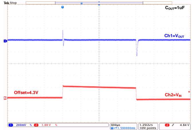
Line Transient at V_{OUT}=3.3V : ( I_{OUT}=10mA )
