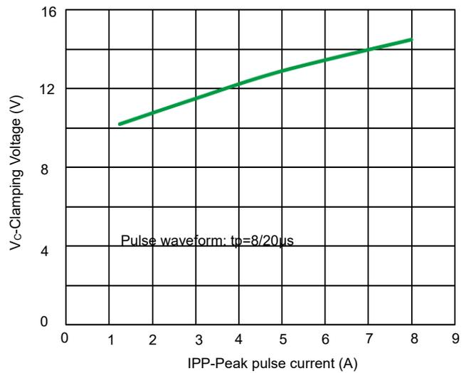
Fig 4. Clamping voltage vs. Peak pulse current
