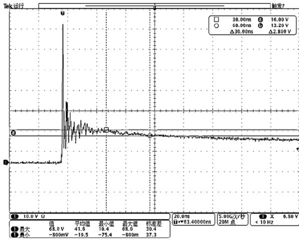
Fig 7. ESD clamping voltage
