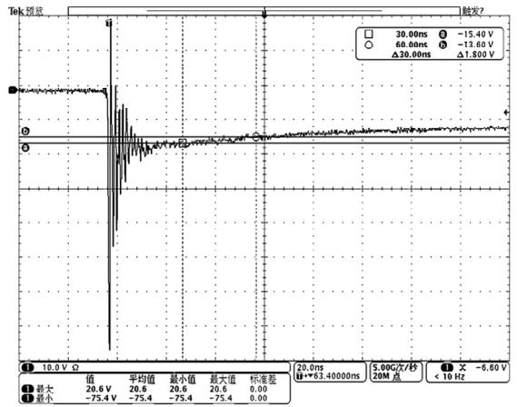
Fig 8. ESD clamping voltage
