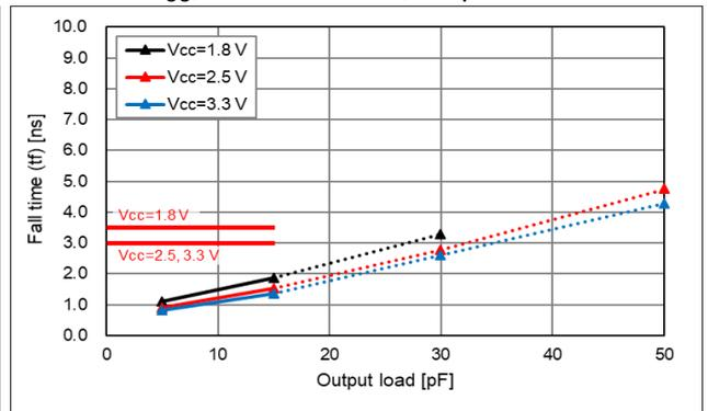
10% - 90% V<sub>CC</sub>, L<sub>CMOS</sub> = 15 pF, Temp. Char.
