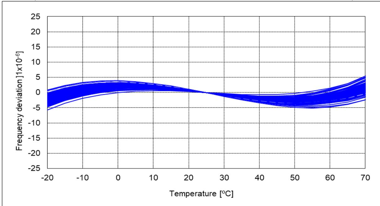
$f_0 = 25 \text{ MHz}$ ,  $\pm 50 \times 10^{-6}$  at  $-40$  to  $+85$  °C/ $+105$  °C
