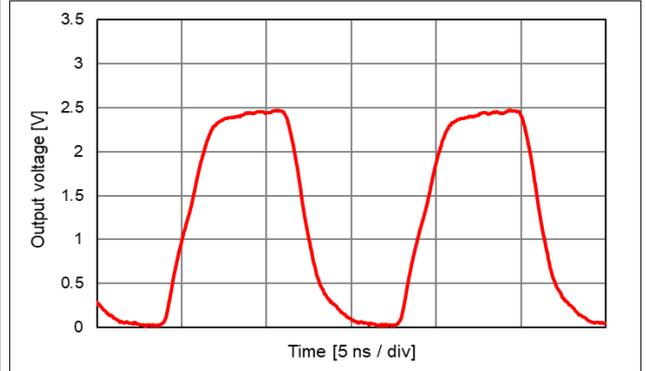
$V_{CC} = 1.8 \text{ V}$ ,  $L_{CMOS} = 15 \text{ pF}$ ,  $T_{use} = +25 \text{ }^\circ\text{C}$
