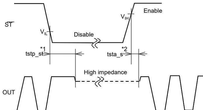
\*1 The period from  $\overline{ST} = V_{IL}$  to  $OUT = High\ impedance\ (Disable)$
