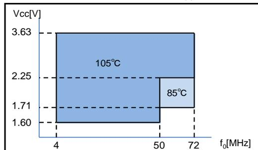
Please note that Supply voltage range (V<sub>CC</sub>) depends on Output frequency(f<sub>o</sub>) and upper limit of Operating temperature(T<sub>use</sub> Max.).
