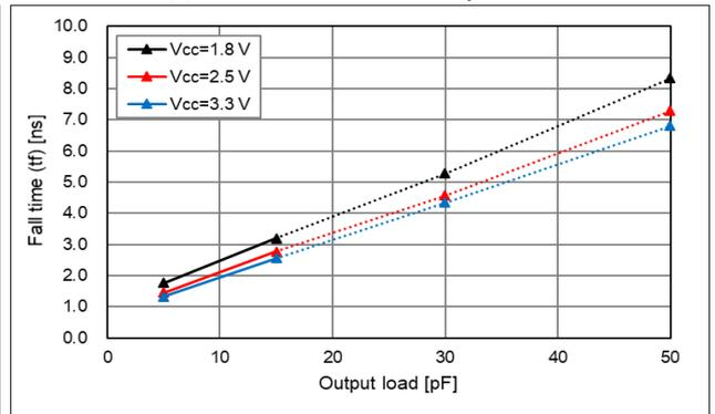
\* Output load condition under L<sub>CMOS</sub> > 15 pF (dotted line area) is not guaranteed, and the data is for reference.
