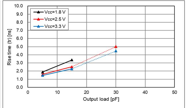
\* Output load condition under L<sub>CMOS</sub> > 15 pF (dotted line area) is not guaranteed, and the data is for reference. There are some missing data in the graph. It is unmeasurable because of low amplitude under the condition of L<sub>CMOS</sub> > 15 pF.
