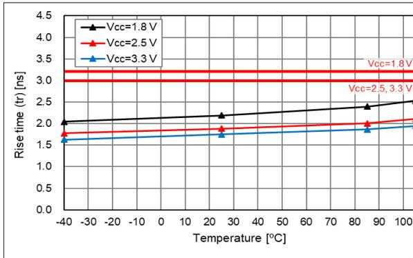
20% - 80% V<sub>CC</sub>, T<sub>use</sub> = +25 °C, Output load Char.
