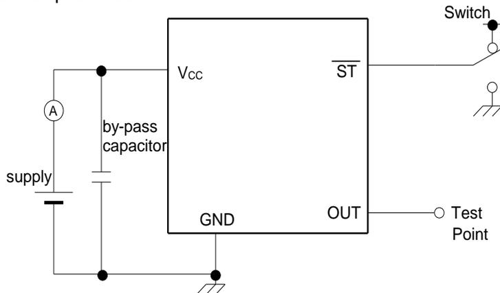
\*Standby current test should be  $\overline{ST} = \text{GND}$ .
