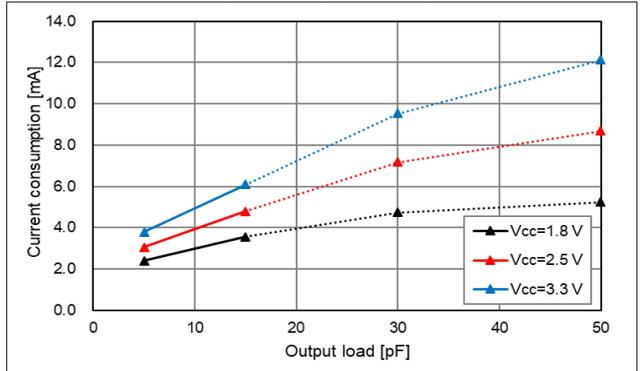
\* Output load condition under  $L_{CMOS} > 15\text{ pF}$  (dotted line area) is not guaranteed, and the data is for reference.
