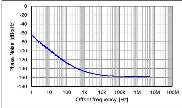
Phase Jitter (Offset frequency: 12 kHz to 5 MHz)
