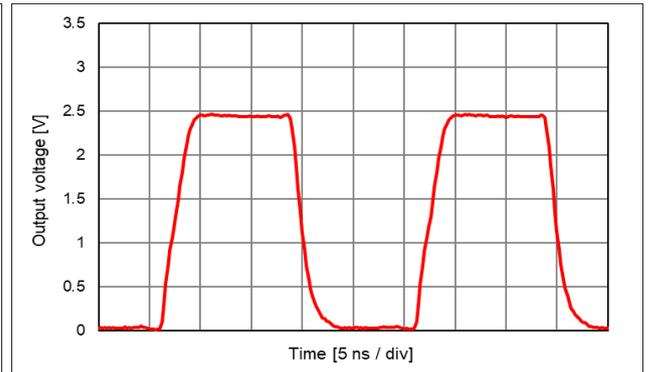
$V_{CC} = 1.8 \text{ V}, L_{CMOS} = 15 \text{ pF}, T_{use} = +25 \text{ }^\circ\text{C}$
