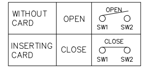
Circuit Diagram for Detect Switch
