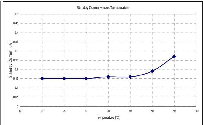
$I_{SD}$  versus Temperature @ VDD = 2.8V, Halogen
