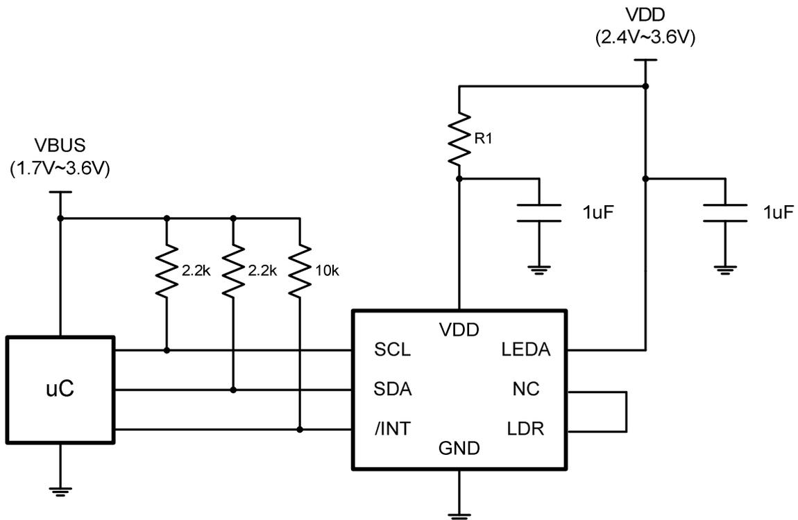
STK3311-WV Typical Application Circuit with Only One Supply Voltage
