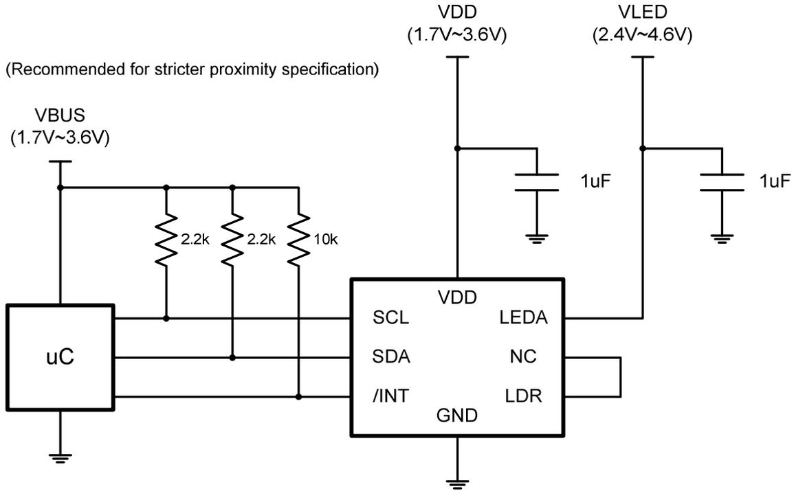
STK3311-WV Typical Application Circuit with Independent VDD and VLED Supply Voltage
