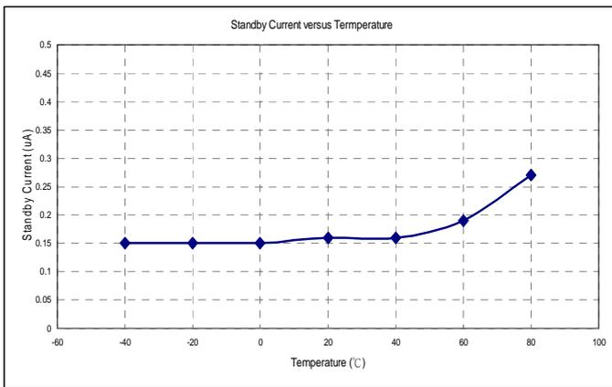
$I_{SD}$  versus Temperature @ VDD = 2.8V, Halogen
