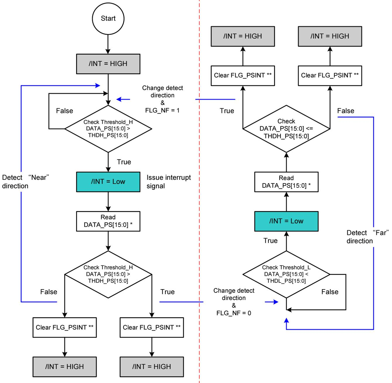
Note : \* read DATA\_PS is driver's behavior and it will trigger IC's next action.
