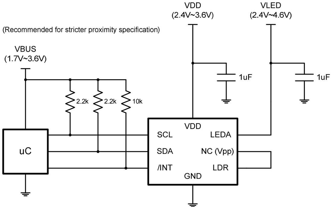
STK3321 Typical Application Circuit with Independent VDD and VLED Supply Voltage
