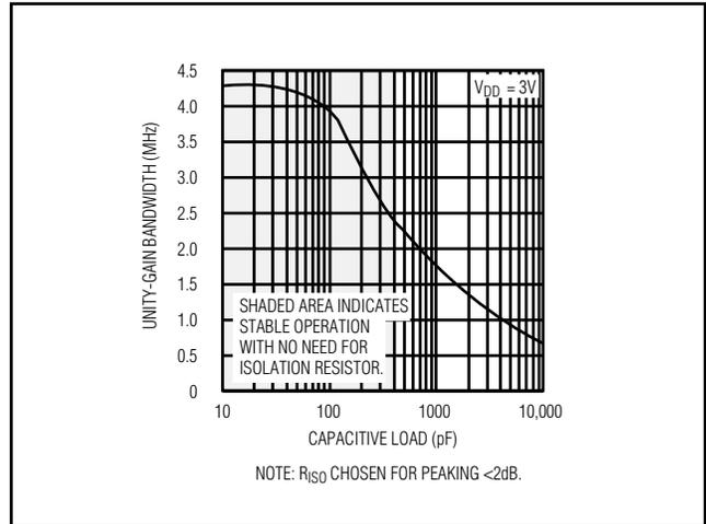
Figure 8. MAX4250–MAX4254 Unity-Gain Bandwidth vs. Capacitive Load
