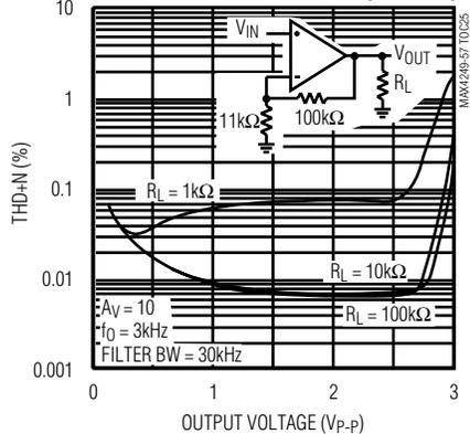
**MAX4249/MAX4255/MAX4256/MAX4257 TOTAL HARMONIC DISTORTION PLUS NOISE vs. OUTPUT VOLTAGE SWING**
