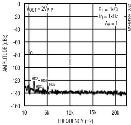
**MAX4249/MAX4255/MAX4256/MAX4257 FFT OF DISTORTION AND NOISE**
