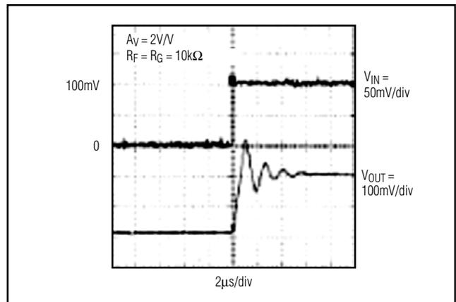
Figure 2a. Pulse Response with No Feed-Forward Compensation
