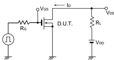
Fig.8 Switching time measurement circuit
