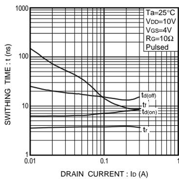
Fig.7 Switching characteristics
