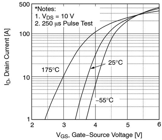
Figure 2. Transfer Characteristics
