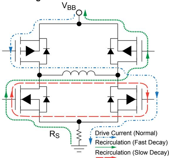
The user selects an external resistor ( $R_T$ ) and capacitor ( $C_T$ ) to determine the time period ( $t_{OFF} = R_T \times C_T$ ) during which the drivers remain disabled (see RC Fixed Off-Time section, below). At the end of the RC interval, the drivers are enabled allowing the load current to increase again. The PWM cycle repeats, maintaining the peak load current at the desired value (figure 2).
