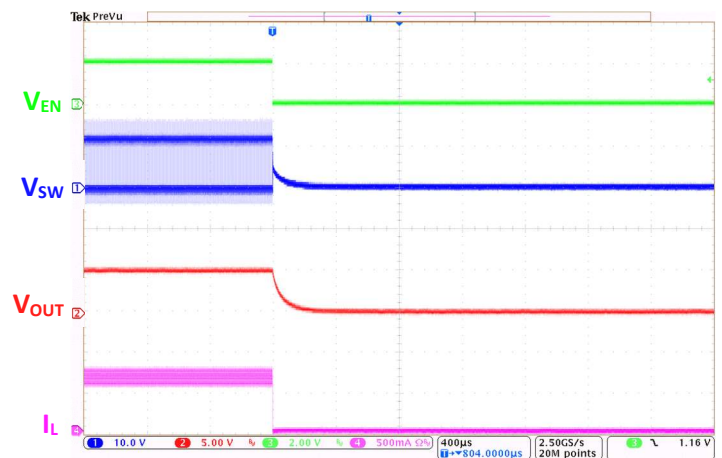
Figure 16. Shutdown Through EN, I_{OUT} = 0.6A
