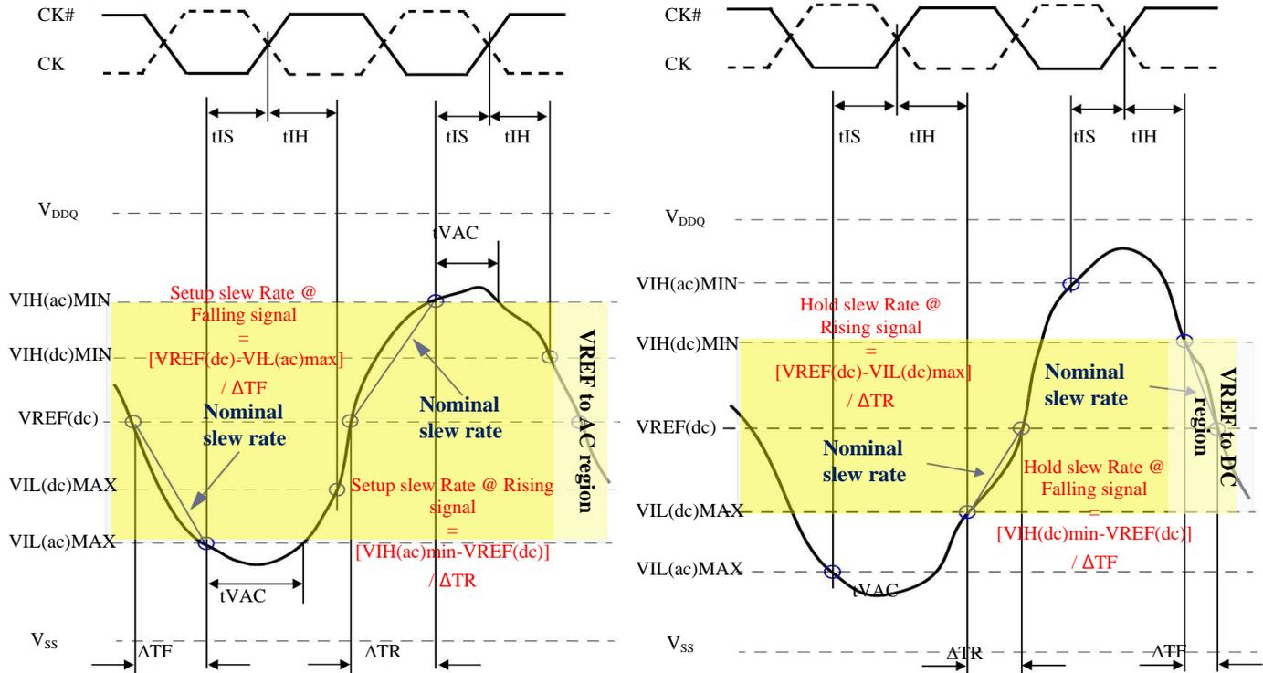
9.5.10.2 Tangent line for setup time tIS(left) and hold time tIH(right) - ADD/CMD with respect to clock
