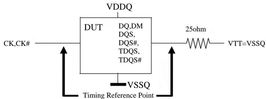
Figure 5.9.1 ODT Timing Reference Load
