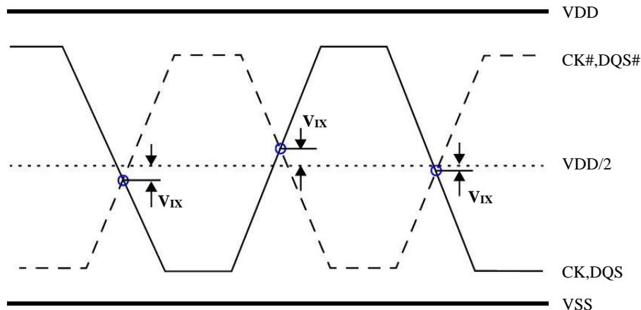
Figure 4.4.  $V_{ix}$  Definition
