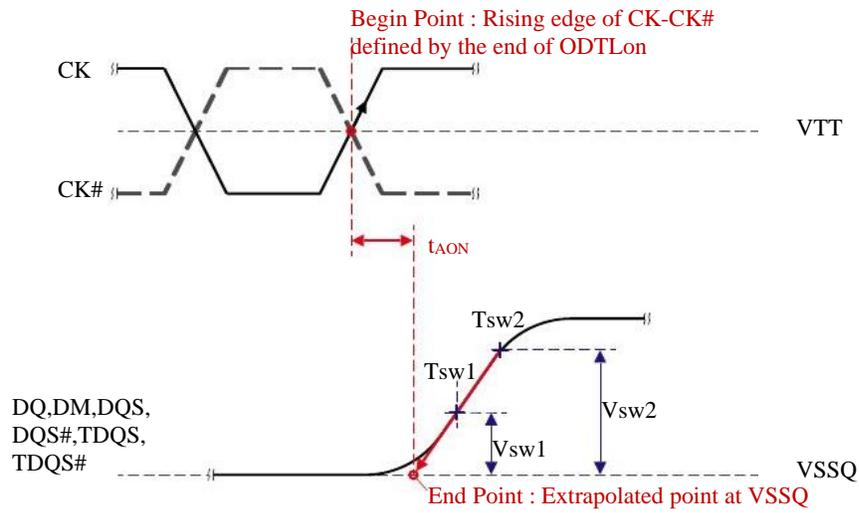
Figure 5.9.2.2 Definition of  $t_{AONPD}$
