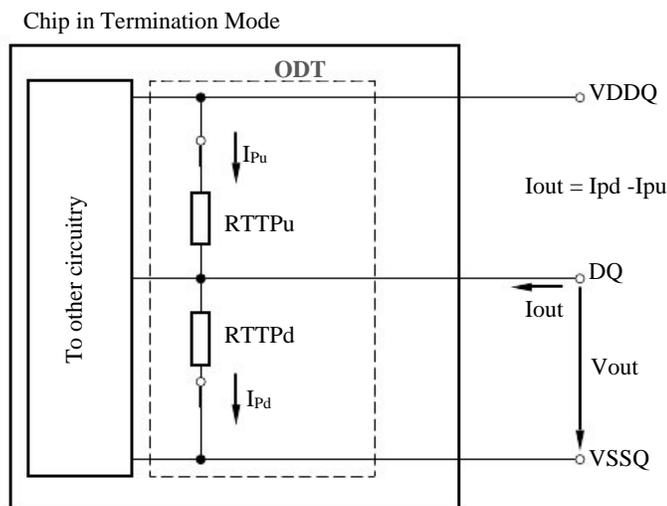
Figure 5.8.1 On-Die Termination : Definition of Voltages and Currents
