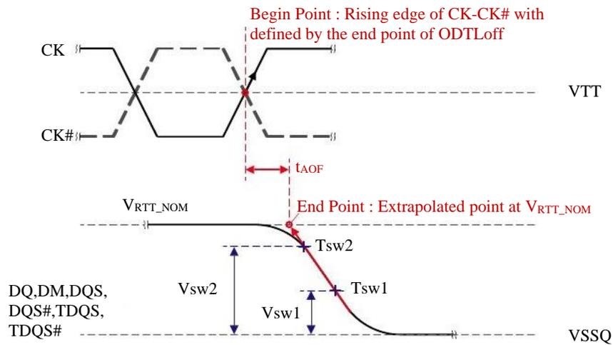
Figure 5.9.2.4 Definition of  $t_{AOFPD}$
