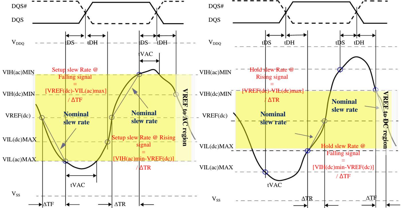
9.6.10.2 Tangent line for setup time tDS(left) and hold time tDH(right) - DQ with respect to strobe
