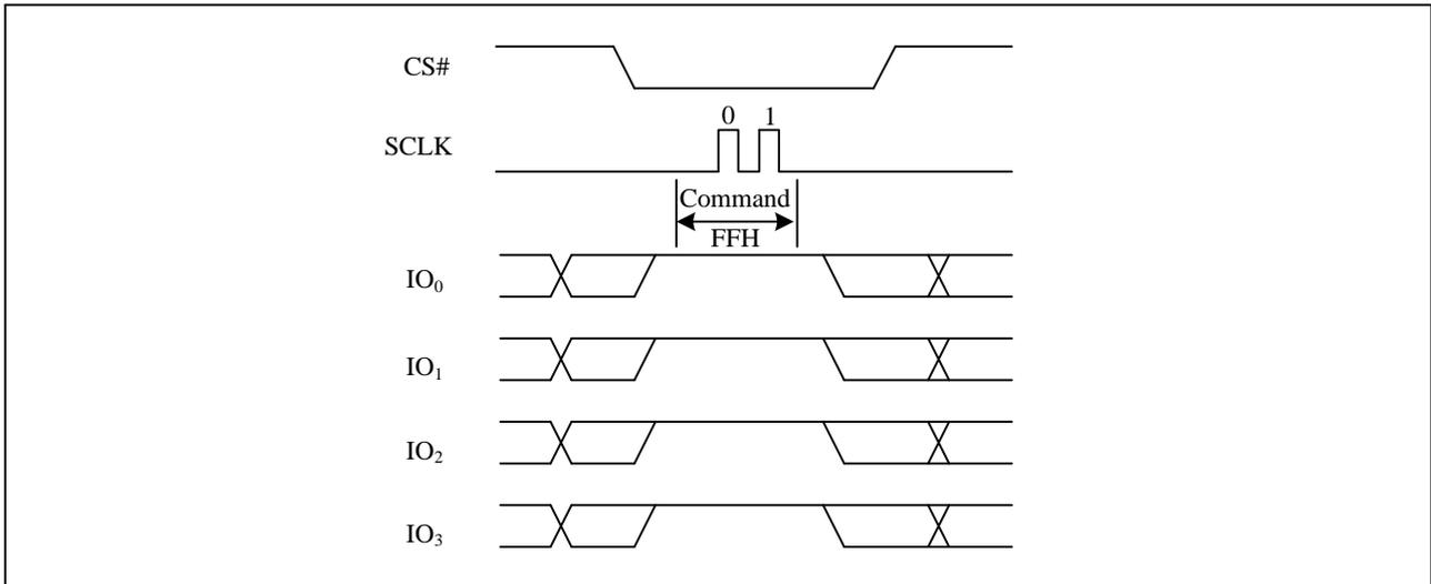
**7.36. Enable Reset (66H) and Reset (99H)**
