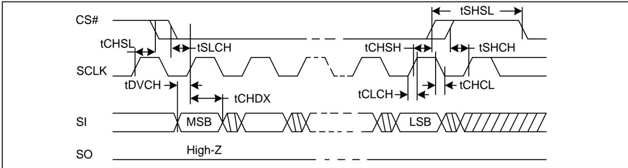
**Figure45. Output Timing**
