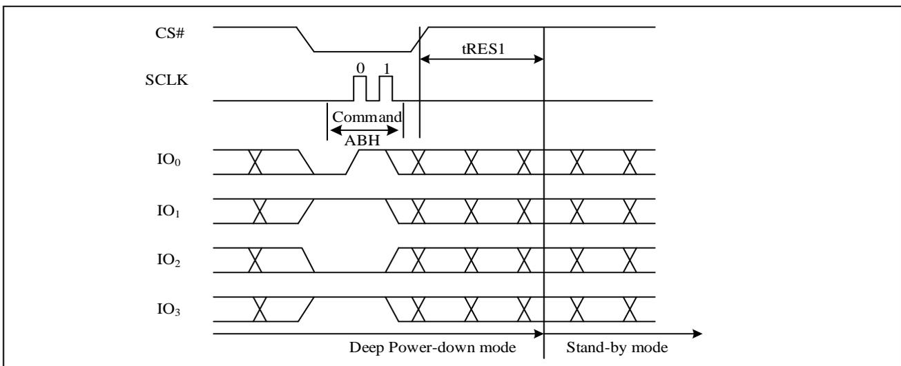
Figure23. Release Power-Down/Read Device ID Sequence Diagram
