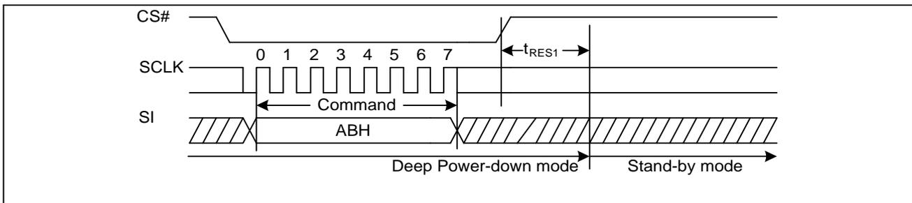
**Figure22a. Release Power-Down Sequence Diagram (QPI)**
