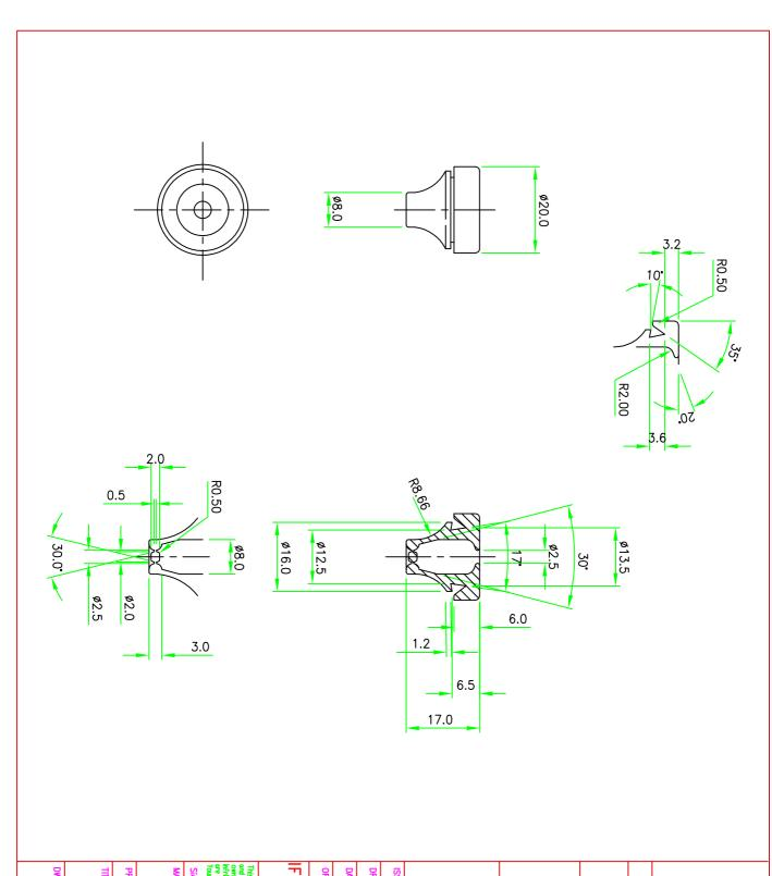
2. EXTERNAL SURFACES TO BE FREE FROM SINK MARKS, PIN HOLES, M/C MARKS, COLOUR VARIATIONS AND OTHER VISIBLE IMPERFECTIONS
