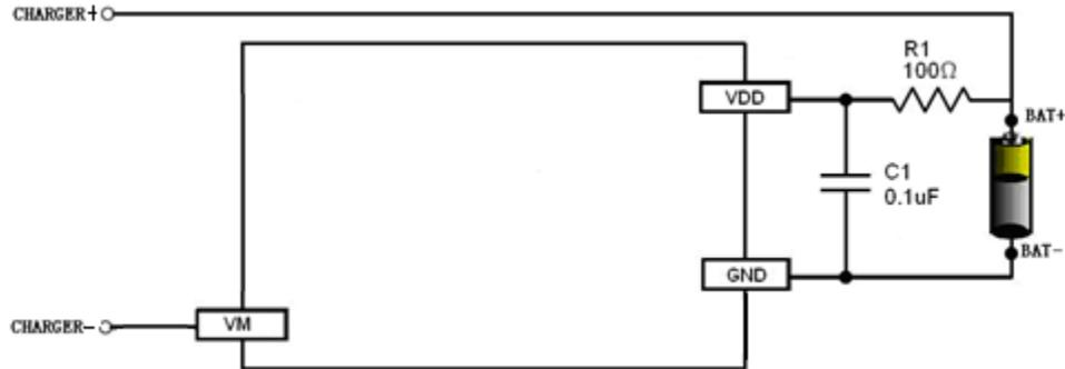
**Fig 6 XB3306D in a Typical Battery Protection Circuit**
