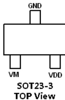
Figure 2. PIN Configuration
