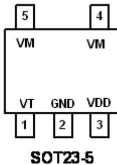
Figure 2. PIN Configuration
