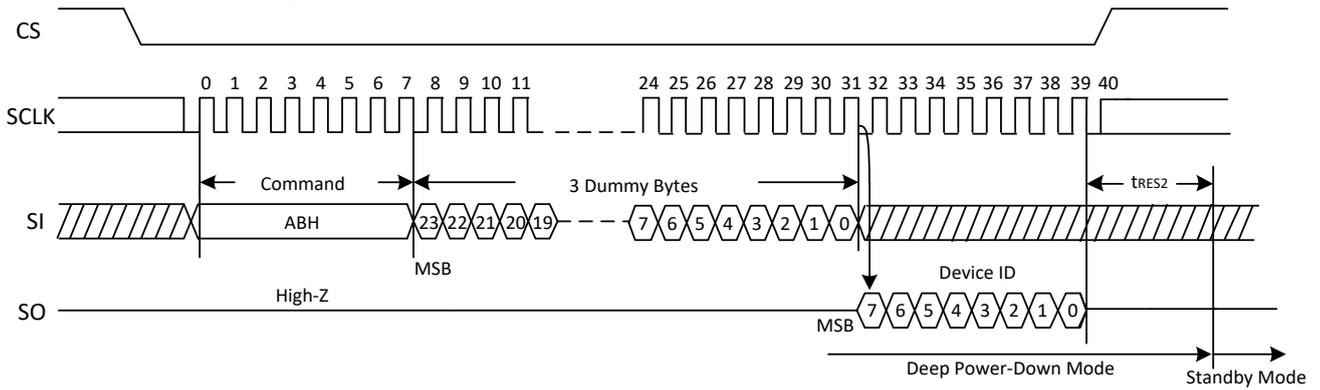
Figure 30c. Release Power-Down/Read Device ID Sequence Diagram (QPI)
