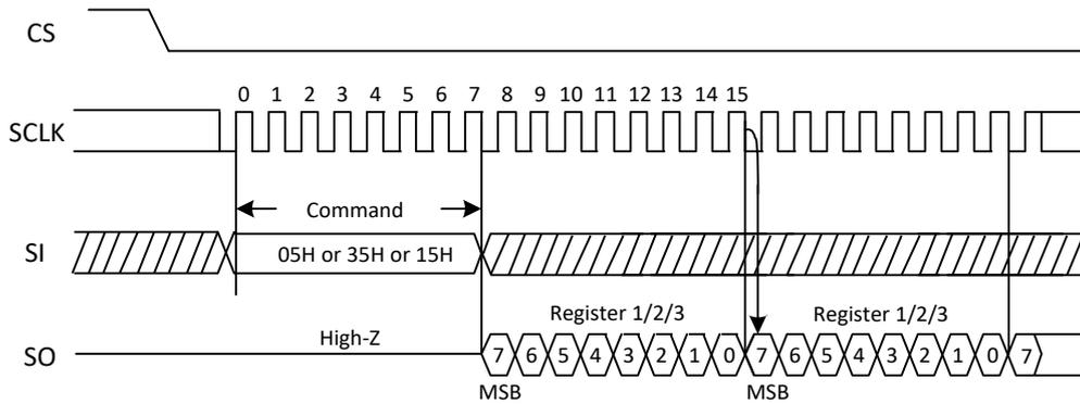
Figure 27a. Read Status Register Sequence Diagram (QPI)
