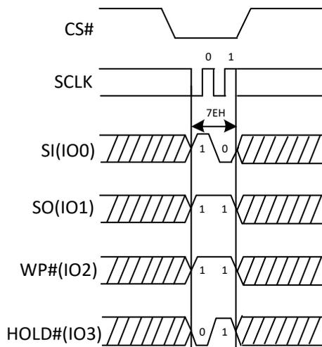
Figure 39b. The Global Block/Sector Unlock Sequence Diagram
