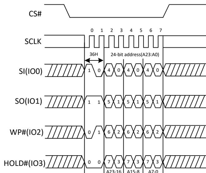
Figure 38b. Individual Block/Sector Unlock command Sequence Diagram
