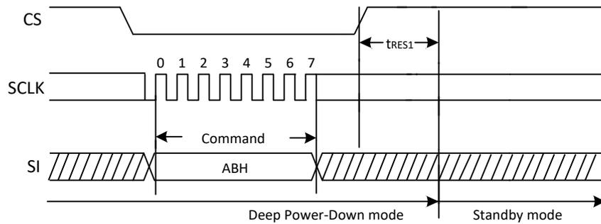
Figure 30a. Release Power-Down Sequence Diagram (QPI)
