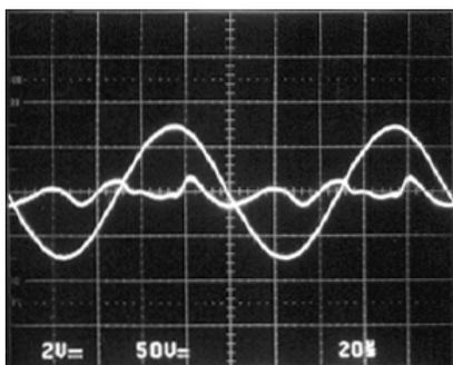
Figure 15. 0.3% THD at 10kHz,  $P_O = 350W$ ,  $R_L = 8\Omega$
