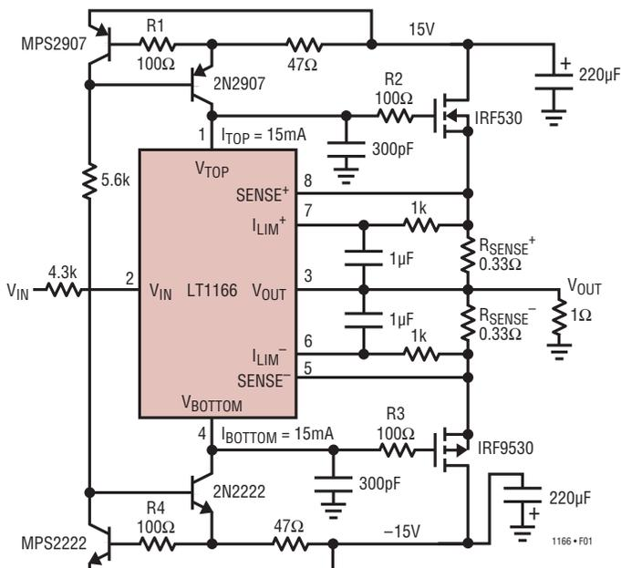
Figure 1. Unity Gain Buffer with Current Limit
