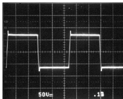
Figure 17. 2kHz Square-Wave,  $C_L = 1\mu F$
