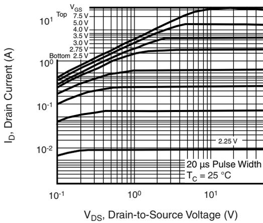
**Fig. 1 - Typical Output Characteristics,  $T_C = 25\text{ }^\circ\text{C}$**
