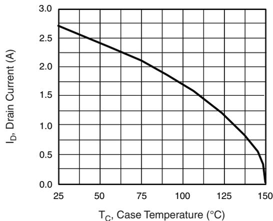
**Fig. 9 - Maximum Drain Current vs. Case Temperature**
