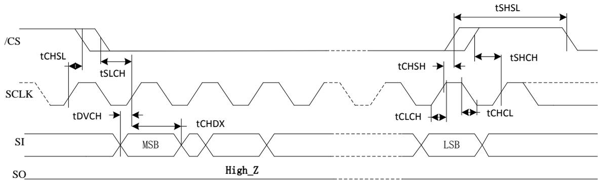
**Figure 37. Output Timing**
