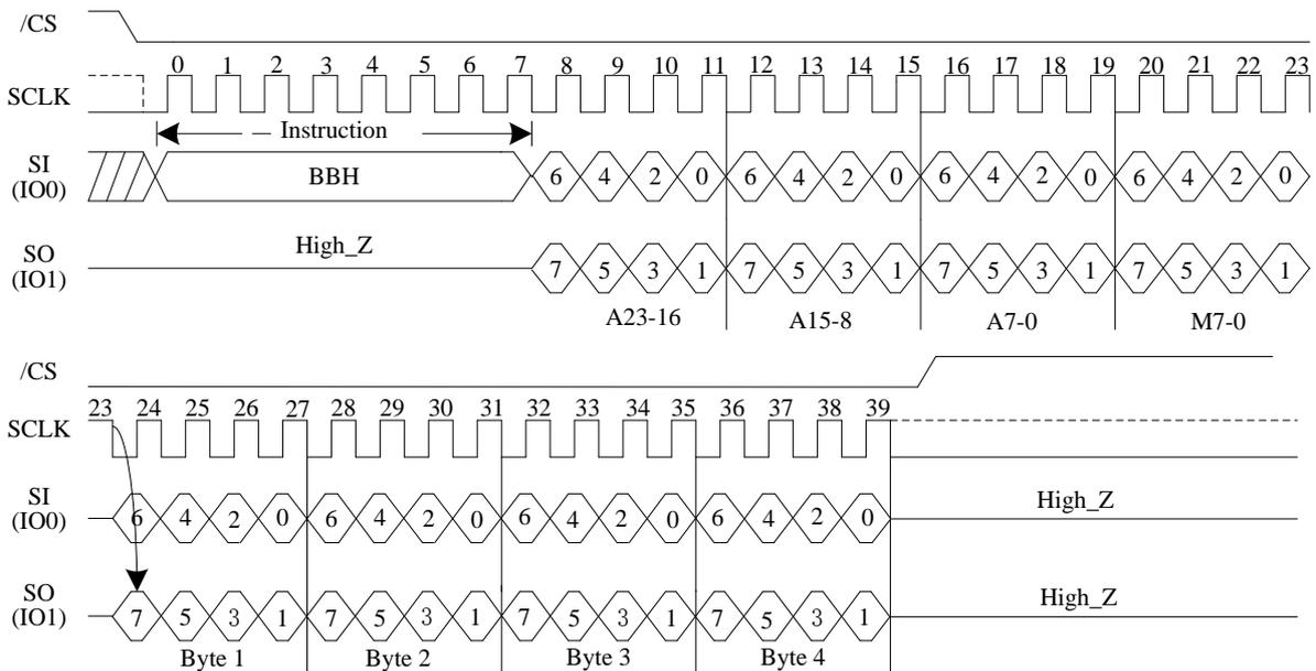
**7.2.6 Dual I/O Fast Read with “Continuous Read Mode”**
