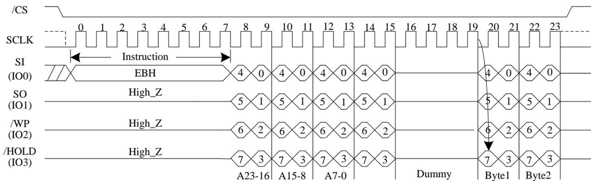
**7.2.8 Quad I/O Fast Read with “Continuous Read Mode”**
