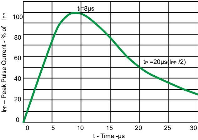
Fig 1. Pulse Waveform
