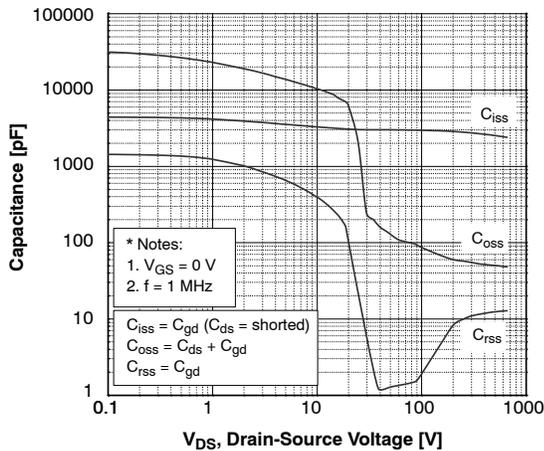
Figure 5. Capacitance Characteristics
