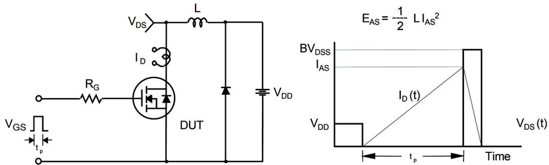
Figure 15. Unclamped Inductive Switching Test Circuit & Waveforms
