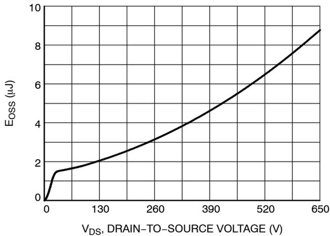
**Figure 11. E<sub>OSS</sub> vs. Drain-to-Source Voltage**
