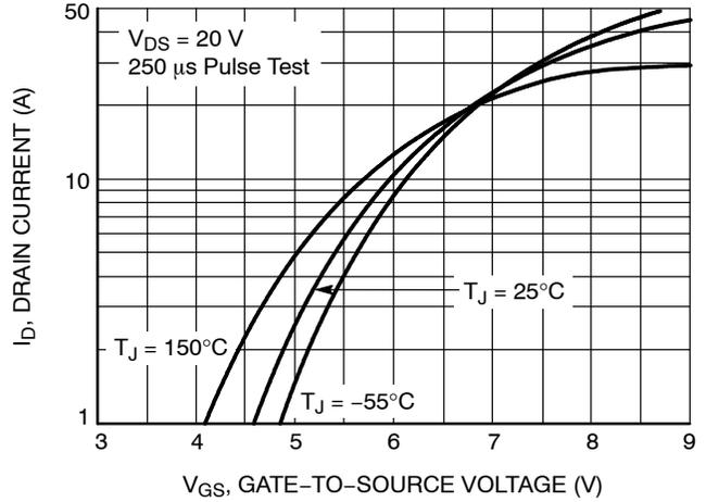
Figure 2. Transfer Characteristics
