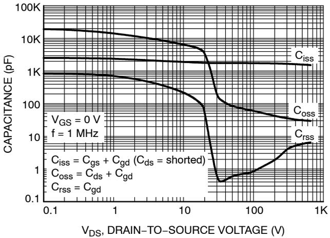
Figure 5. Capacitance Characteristics
