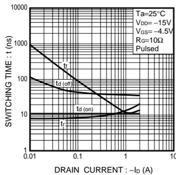
Fig.8 Switching Characteristics
