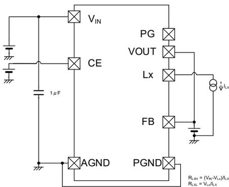
$R_{Lx} = (V_{IN} - V_{OUT}) / I_{Lx}$
