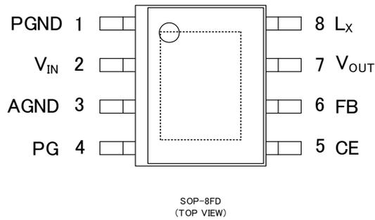
\* The dissipation pad for the SOP-8FD package should be solder-plated in recommended mount pattern and metal masking so as to enhance mounting strength and heat release. If the pad needs to be connected to other pins, it should be connected to the GND (No.1,3) pin.
