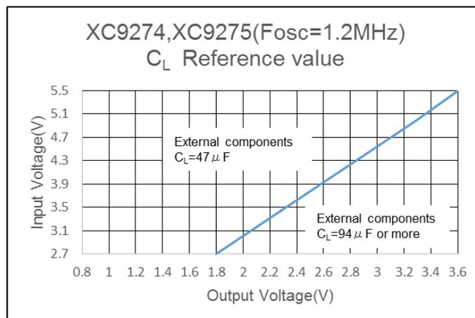
Fig.1:XC9274, XC9275 ( $f_{osc}=1.2\text{MHz}$ ) C<sub>L</sub> Value
