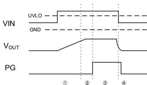
①When a voltage which is higher than UVLO release voltage is fed to VIN then the output voltage goes up with a soft-start function. During the soft-start, PG goes down to GND level and stays at the level.
