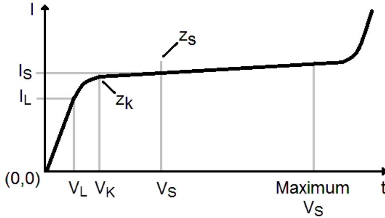
FIGURE 1 – CURRENT-REGULATOR CHARACTERISTICS
