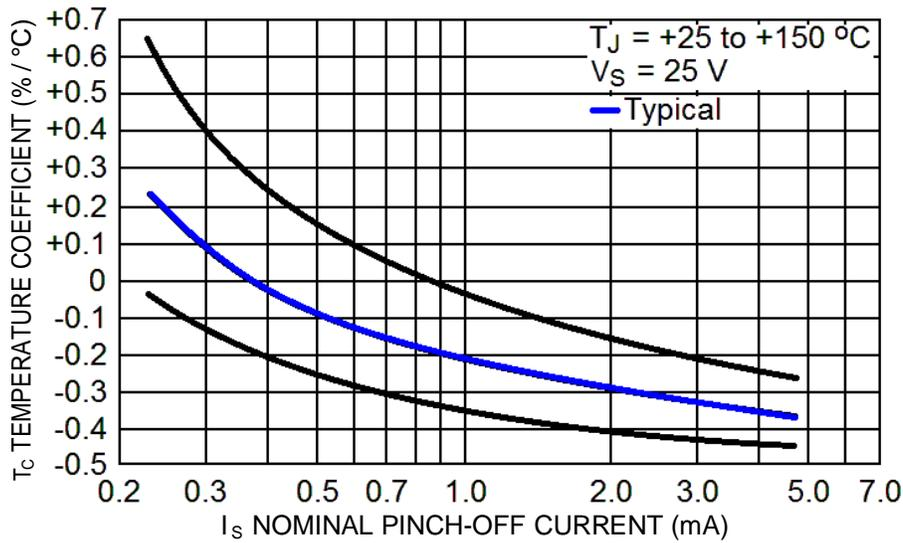
FIGURE 2 – TEMPERATURE COEFFICIENT
