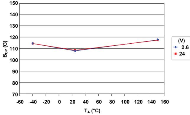
Operate Point versus Supply Voltage
