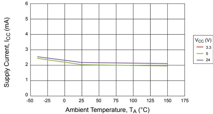
Supply Current (Off) versus Ambient Temperature
