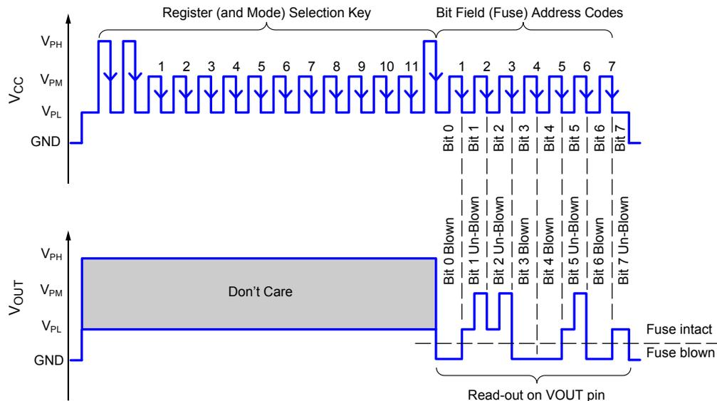
Figure 9. Read mode example. Pulse sequence for accessing the  $B_{OP}$  Selection register (BOPSEL) and reading back the status of each of the eight bit fields. In this example, the code (blown fuses) is  $2^0 + 2^3 + 2^4 + 2^6 = 89$  (0101 1001). After each address pulse is sent, the voltage on the VOUT pin will be at GND for blown fuses and at  $V_{CC}$  (at  $V_{PL}$  or  $V_{PM}$ ) for un-blown fuses.
