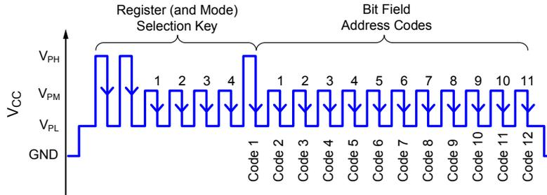
Figure 10. Example of Try mode programming pulses applied to the VCC pin. In this example,  $B_{OP}$  Positive Trim, Down-Counting register is addressed to code 12 by the eleven  $V_{PM}$  pulses (code 1 is selected automatically at the falling edge of the register-mode selection key).
