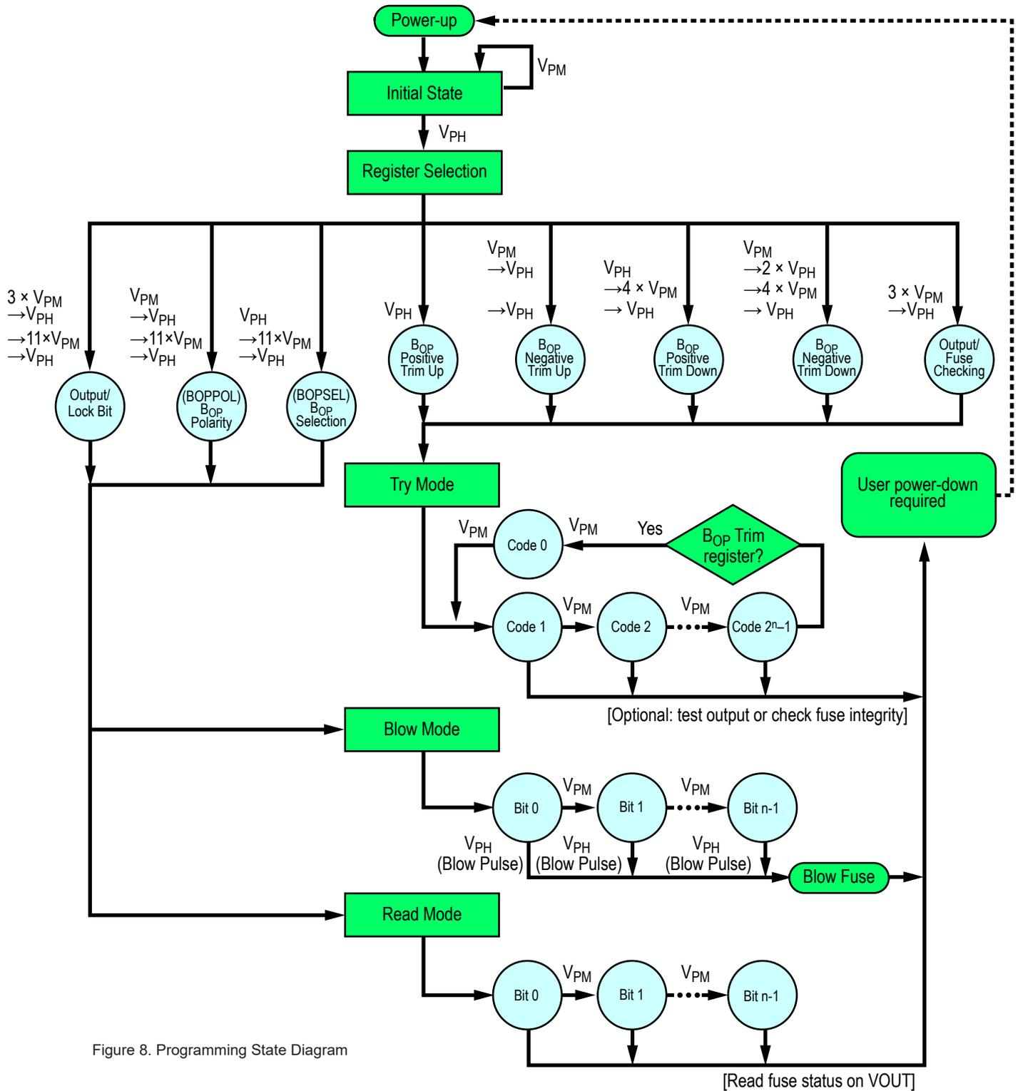
Figure 8. Programming State Diagram
