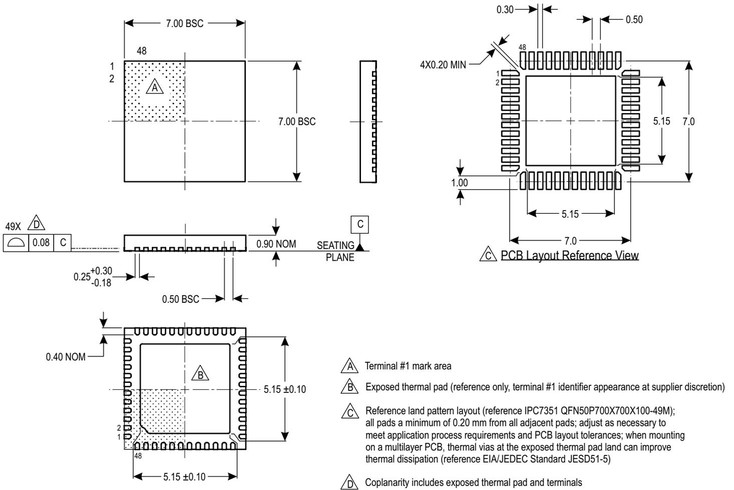
Figure 5: Package EV, 48 Terminal QFN with Exposed Thermal Pad
