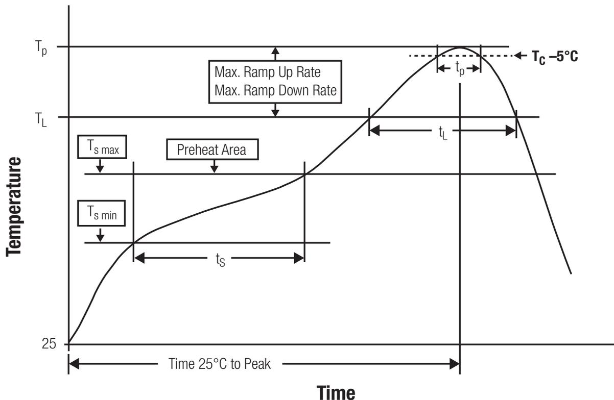
Figure 14: Reflow soldering profile
