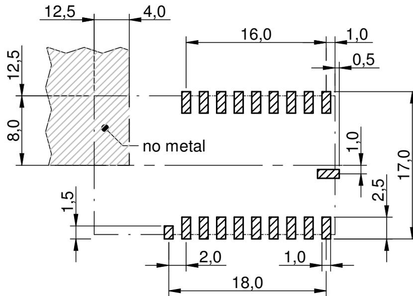
Figure 16: Footprint and dimensions [mm]
