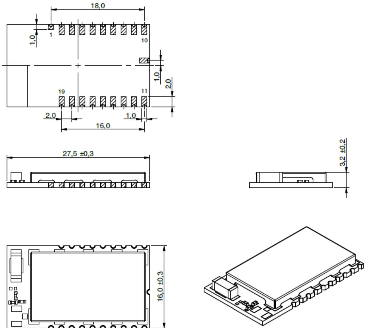
Figure 15: Module dimensions [mm]
