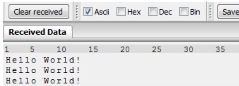
You just used the so called "transparent mode" of the modules to send your data. The address mode that was used is "0". Thus all radio frames are broadcasts that can be received by any other device using the same radio settings. The frame you send was generated using the timeout method.
