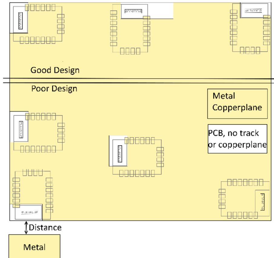
Figure 5: Placement of the module with integrated antenna
