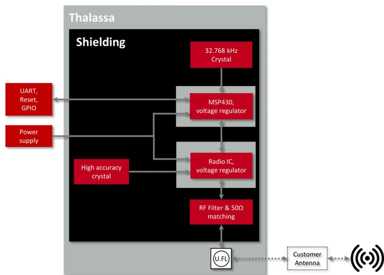
Figure 1: Block diagram of the 3 module variants
