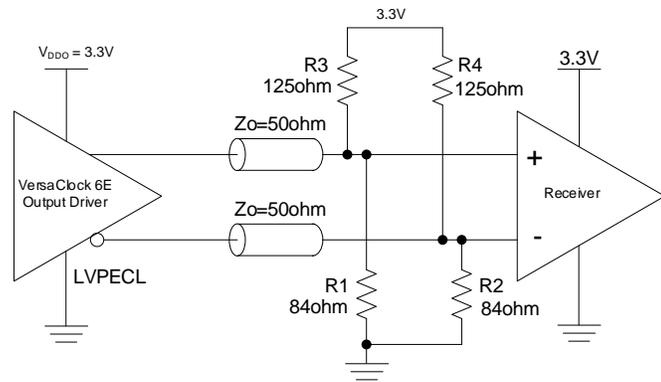
Figure 16. 2.5V LVPECL Output Termination (2)
