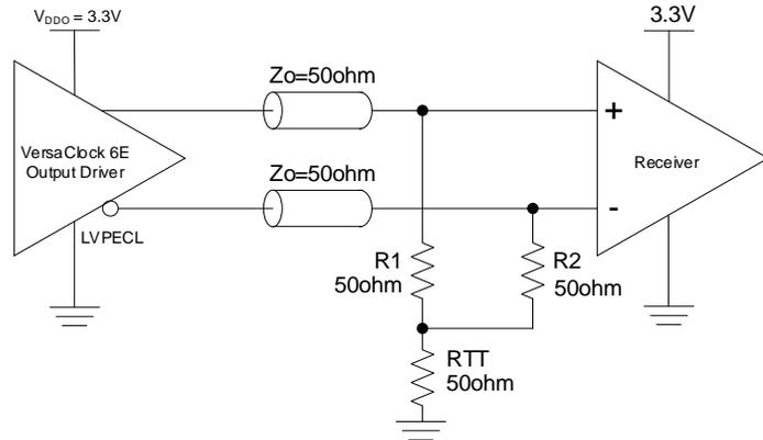
Figure 15. 2.5V LVPECL Output Termination
