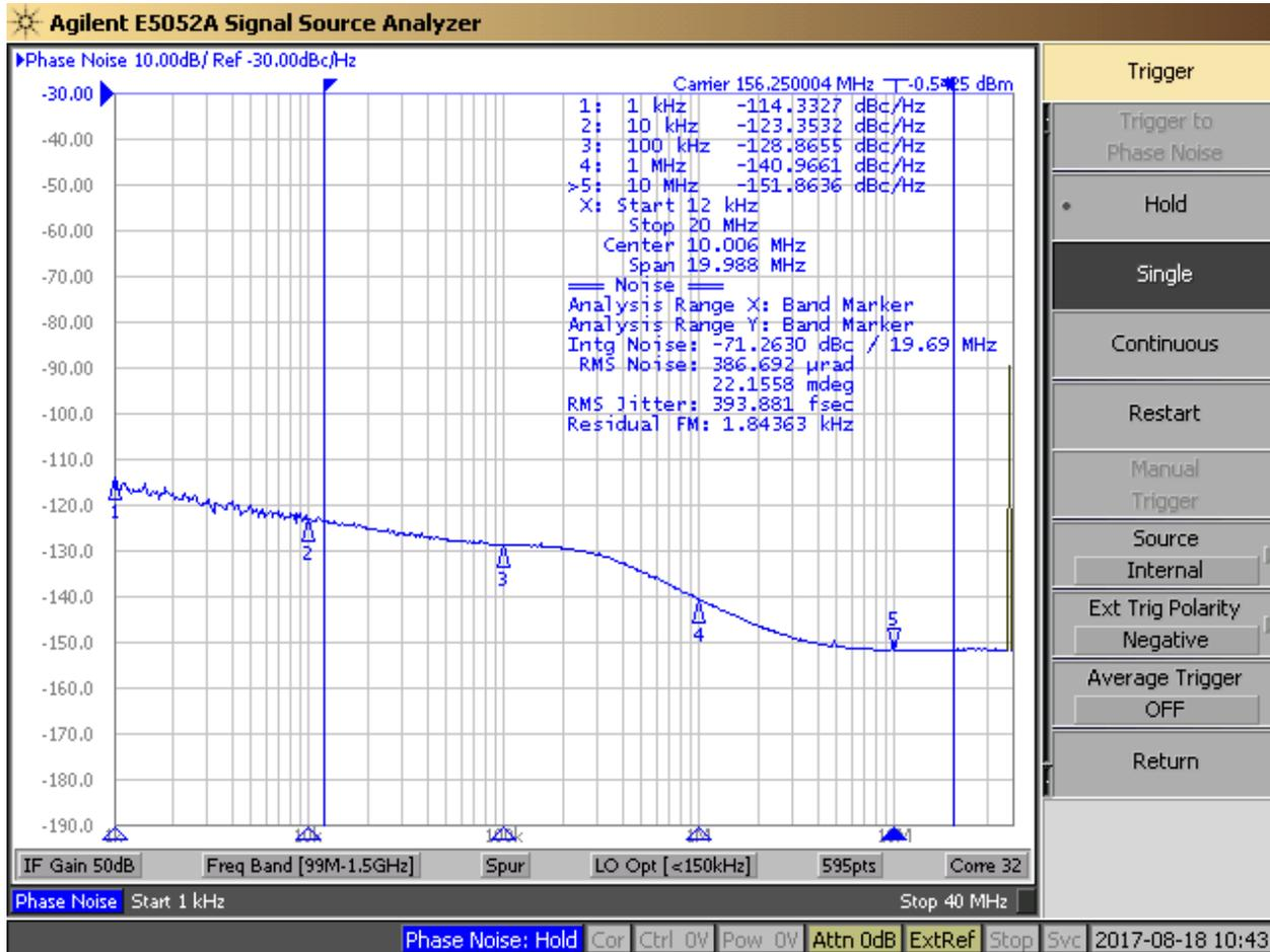
Note: Measured with OUT2=156.25MHz on, 39.625MHz input.
