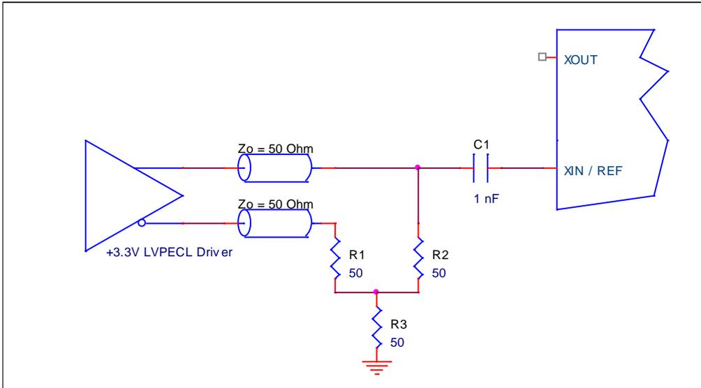
Table 23 shows resistor values that ensure the maximum drive level for the XIN port is not exceeded for all combinations of 5% tolerance on the driver  $V_{DD}$ ,  $V_{DD0}$ , and 5% resistor tolerances. The resistor values can be adjusted to reduce the loading for a slower and weaker LVCMOS driver by increasing the impedance of the R1–R2 divider. To better assist with this assessment, the total load ( $R_0+R_s+R_1+R_2$ ) on the driver is included in the table.
