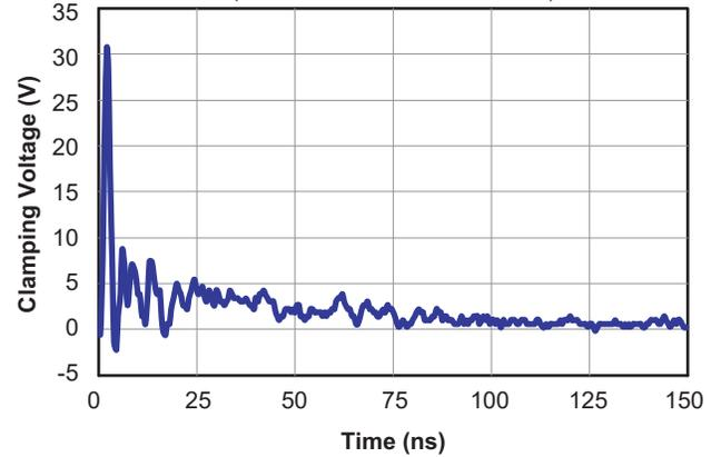
**-8kV ESD Clamping Per IEC 61000-4-2**
