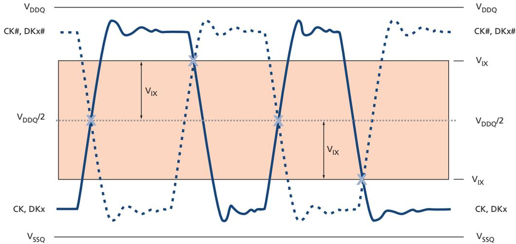
Figure 10: Single-Ended Requirements for Differential Signals
