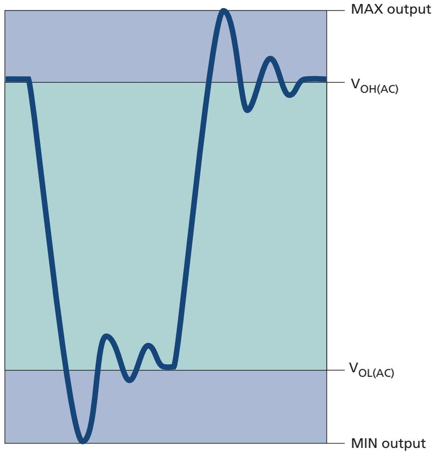
Figure 17: Differential Output Signal
