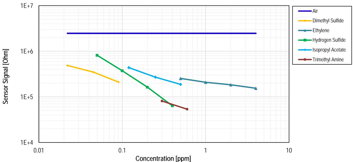
The sensor module outputs are raw resistance measurements and an algorithmic calculation of the refrigeration air quality change (RAQ), which indicates a total air quality change over time inside the refrigeration application. RAQ is a ratio of concentrations and defined as the following:
