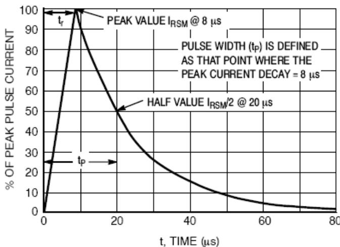
Figure 1. 8 x 20  $\mu\text{s}$  Pulse Waveform
