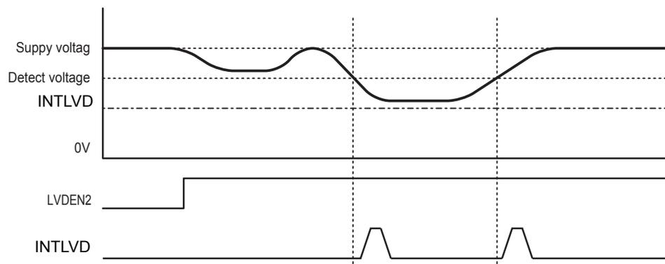
Figure 18-2 low voltage detection Timing
