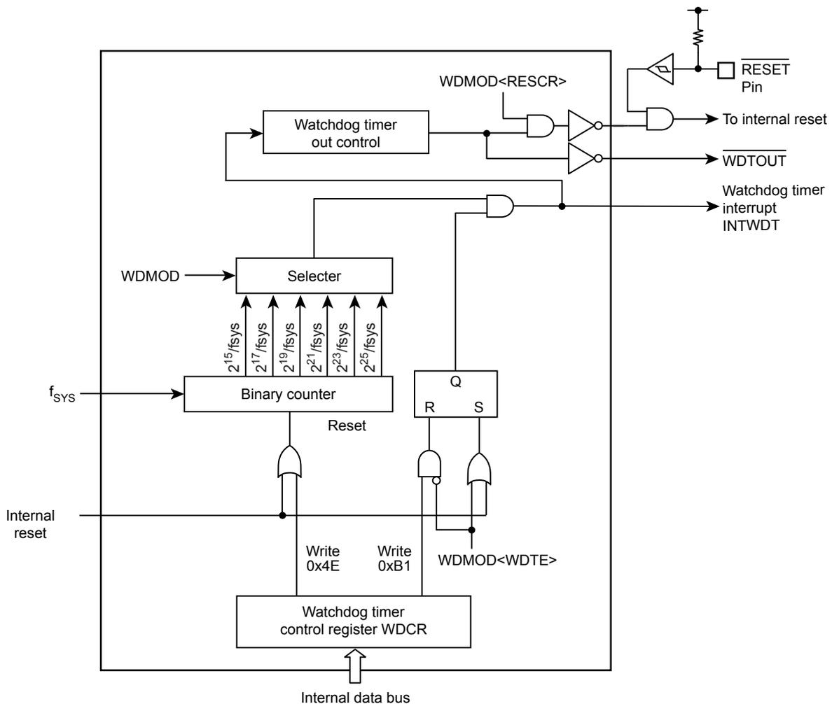
Figure 19-1 Block Diagram of the watchdog Timer
