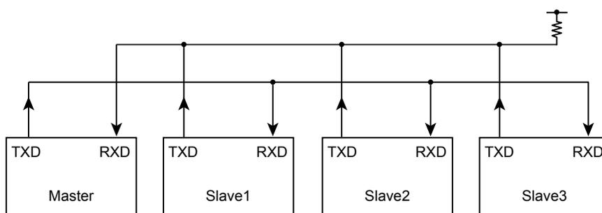
Figure 11-19 Serial Links to Use Wake-up Function
