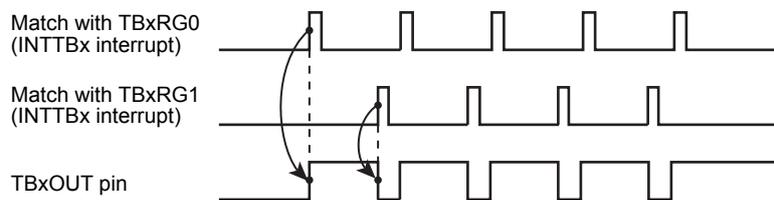
Figure 9-2 Example of Programmable pulse generation output
