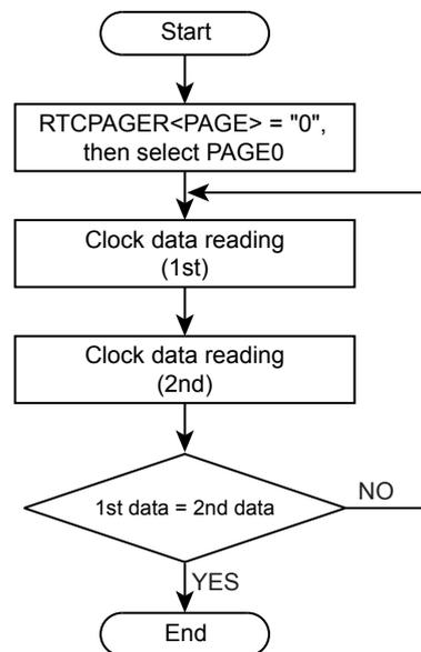
Figure 16-2 Flowchart of the clock data reading
