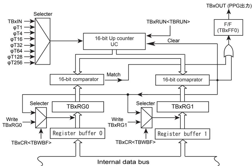
Figure 9-4 Block diagram of 16-bit PPG mode
