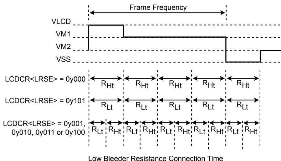
$R_{Lt}$  : Period during which low resistance is connected
