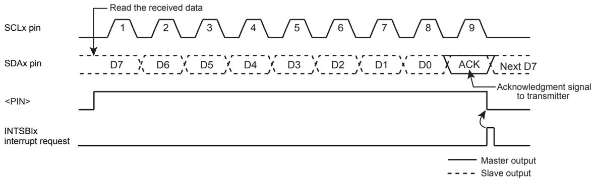
Figure 12-9 <BC[2:0]>= "000", <ACK>= "1" (Receiver Mode)
