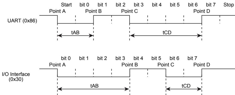
Figure 20-6 Serial operation mode determination data
