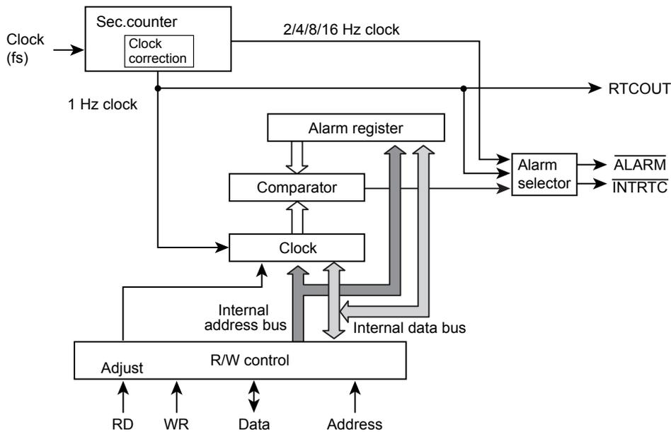
Figure 16-1 Block Diagram
