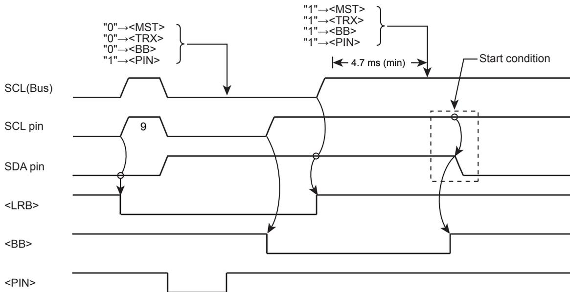
Figure 12-12 Timing Chart of Generating a Restart
