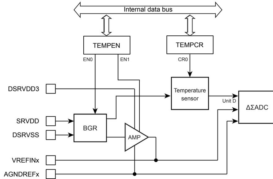
Figure 15-1 Block diagram of Temperature sensor
