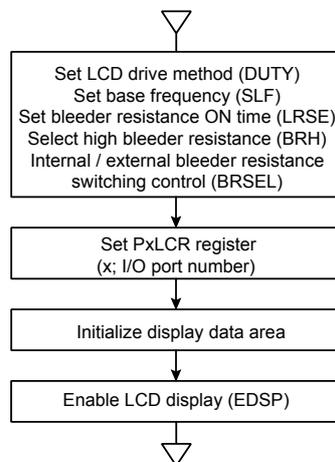
Figure 17-5 Flowchart for the LCD Driver Initialization
