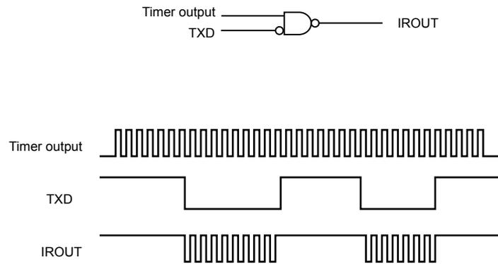
Figure 11-10 Output signal using IR carrier pulse
