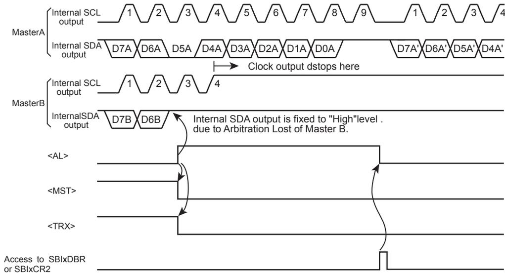
Figure 12-6 Example of Master B Lost Arbitration ( $D7A = D7B$ ,  $D6A = D6B$ )
