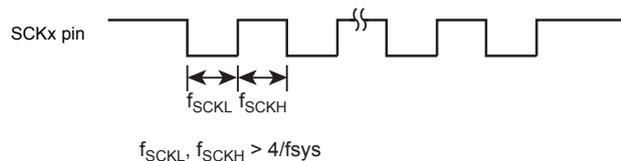
Figure 12-14 Maximum Transfer Frequency of External Clock Input
