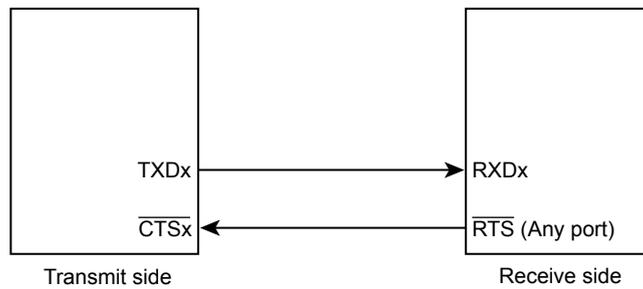
Figure 11-8 Handshake Function
