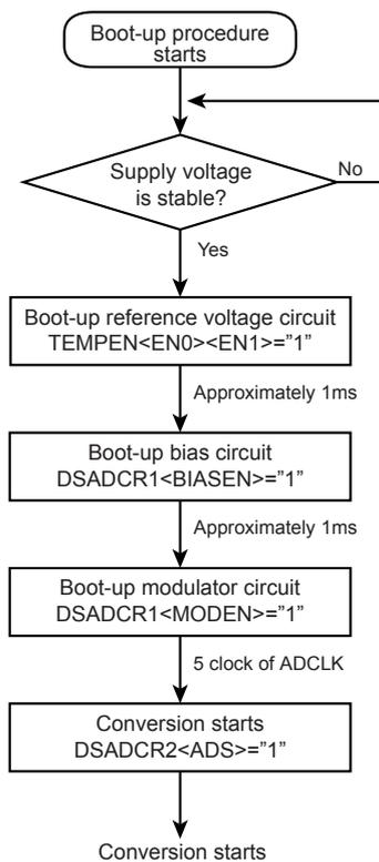
Figure 14-2 Boot-up procedure
