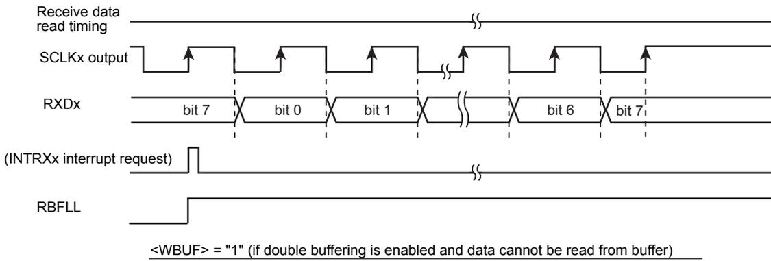
Figure 11-15 Receive Operation in the I/O Interface Mode (SCLK Output Mode)
