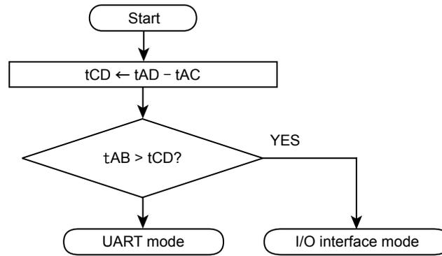
Figure 20-8 Serial operation mode determination flowchart
