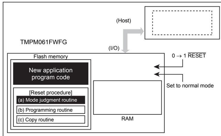
20.4.2 (1-B) Procedure that a Programming Routine is transferred from External Host
