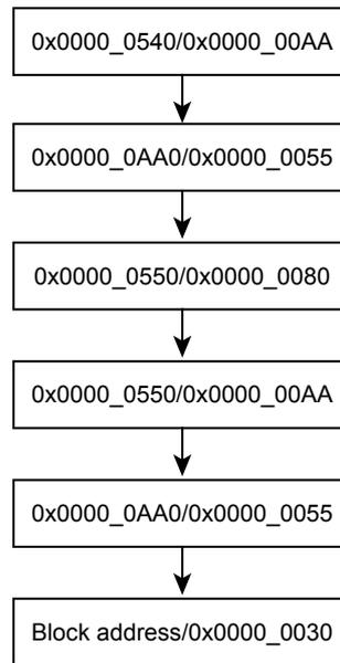
Figure 20-5 Flowchart of automatic erase
