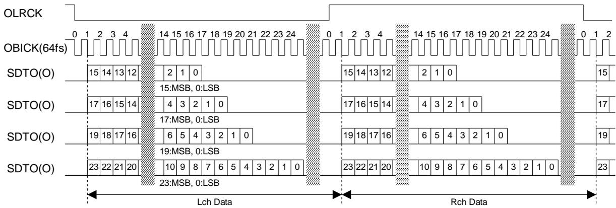
Figure 27. Stereo Mode I<sup>2</sup>S Compatible Timing
