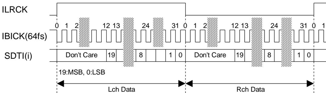
Figure 15. Mode 1 Timing (20bit, LSB justified)
