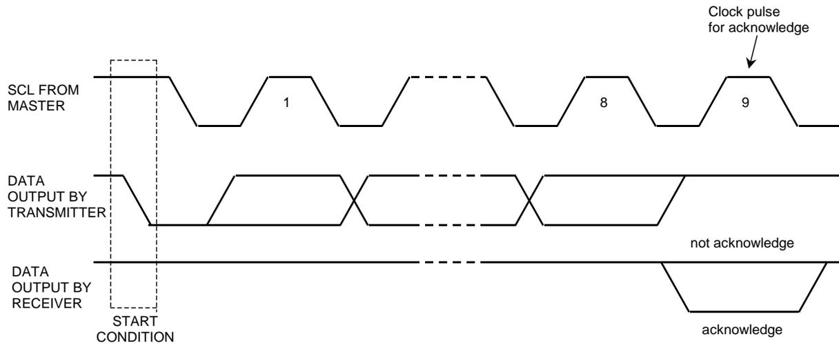
Figure 41. Acknowledge on the I<sup>2</sup>C-bus
