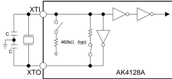
The OMCLK/XTI pin is pulled down when the PDN pin= "L".
