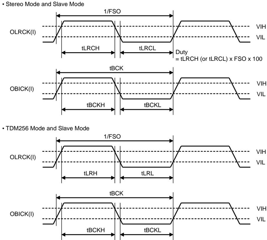
Figure 7. OLRCK, OBICK, Clock Timing (Slave Mode)
