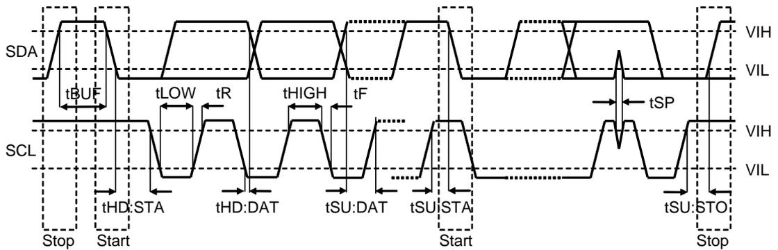
Figure 13. I<sup>2</sup>C Bus Timing
