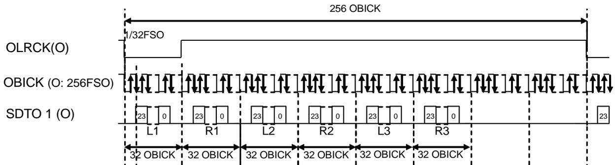
Figure 30. TDM 256 mode 24bit I<sup>2</sup>S Compatible Timing at Master Mode (SDTO2-4: “L” outputs)
