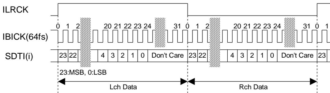
Figure 16. Mode 2 Timing (24bit, MSB justified)
