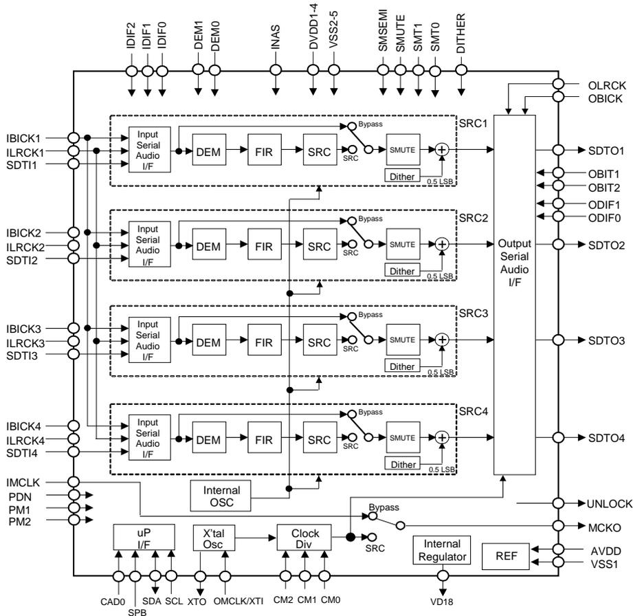
Figure 23. Bypass Mode in Slave Mode (Synchronous mode INAS pin = "L")
