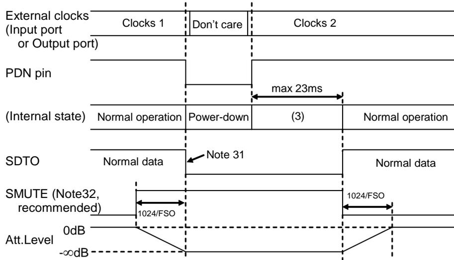
Note 31. The data on SDTO may cause a clicking noise. To prevent this, set “0” to the SDTI more than 1024/fs (GD) before the PDN pin changes to “L”. It makes the data on SDTO remain as “0”.
