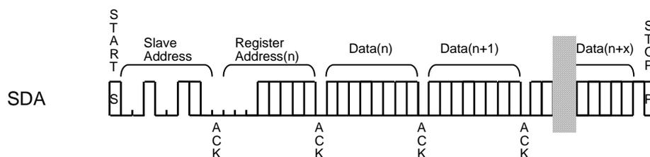
Figure 45. WRITE Operation
