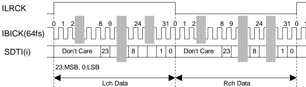
Figure 18. Mode 4 Timing (24bit, LSB justified)
