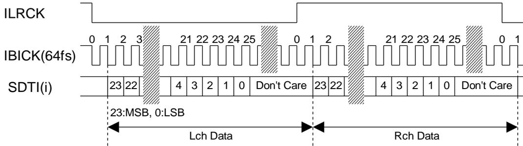
Figure 17. Mode 3 Timing (24bit I<sup>2</sup>S)
