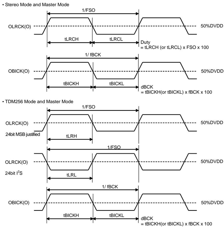
Figure 8. OLRCK, OBICK, Clock Timing (Master Mode)
