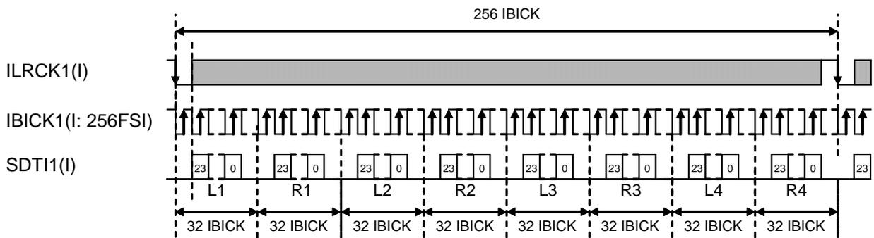
Figure 20. Mode 6 Timing (TDM, I<sup>2</sup>S, SDTI2-4: Don't care)
