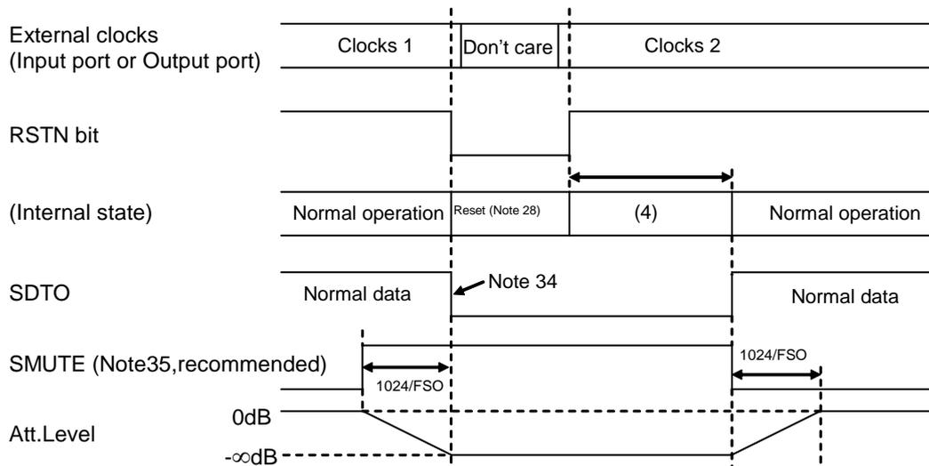
Note 34. The data on SDTO may cause a clicking noise. To prevent this, set “0” to the SDTI from GD before the RSTN pin changes to “L”. It makes the data on SDTO remain as “0”.
