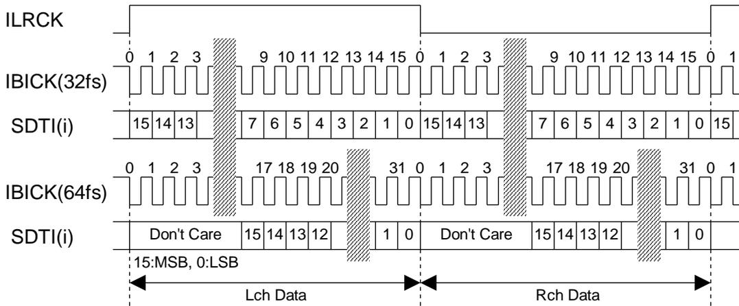
Figure 14. Mode 0 Timing (16bit, LSB justified)
