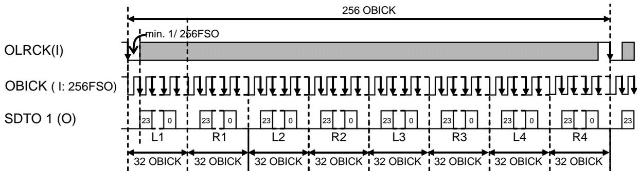
Figure 31. TDM 256 mode 24bit I<sup>2</sup>S Compatible Timing at Slave Mode (SDTO2-4: “L” outputs)
