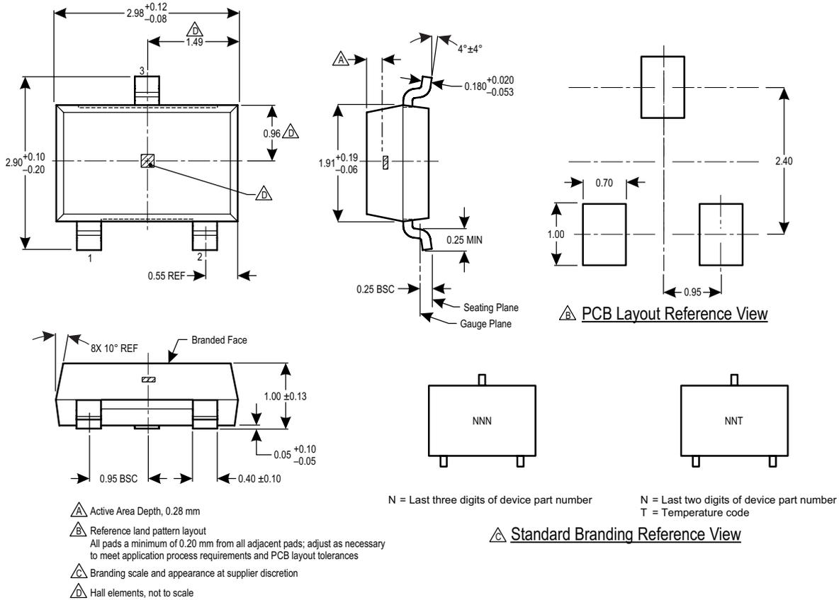
Figure 3: Package LH, 3-Pin SOT-23W
