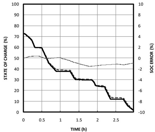
**REAL APPLICATION UNDER CV MODE SOC ACCURACY 1**
