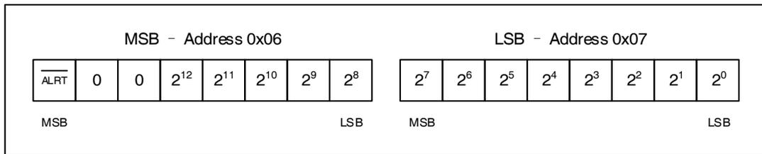
Figure 5. RRT\_ALERT Register Format
