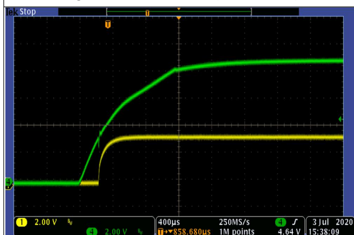
Fig 7 Vout Load Transient (50 to 250mA)
