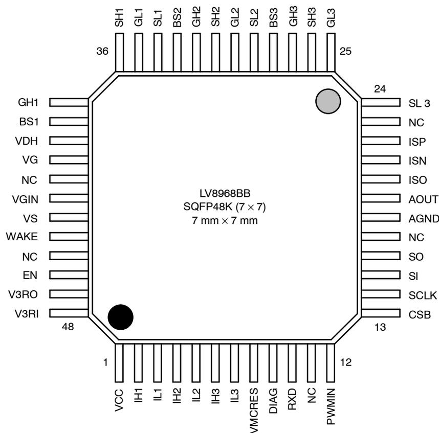
Figure 2. LV8968BB Pinout
