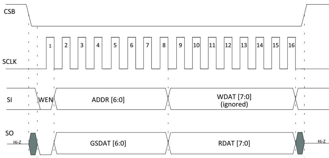
**Figure 9. SPI Format in Read Mode**
