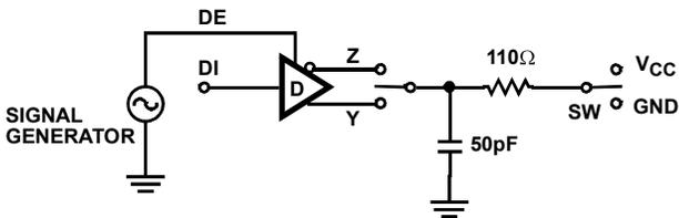
FIGURE 3A. TEST CIRCUIT
