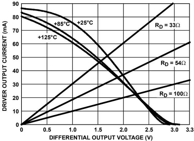
FIGURE 8. DRIVER OUTPUT CURRENT vs DIFFERENTIAL OUTPUT VOLTAGE
