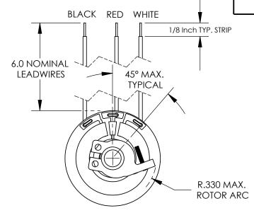
$.045 \pm .005$ Ø.186<sup>+.002</sup><sub>-.005</sub> .075 REF. ELEMENT I.D. Ø.702±.002 ELEMENT O.D. Ø.125<sup>+.004</sup>-.000 INSULATOR I.D. .075 +.005 .200 REF.
