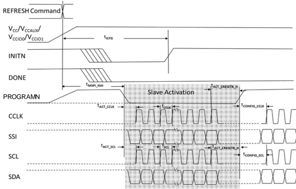
Figure 3.15. Slave SPI/I<sup>2</sup>C/I<sup>3</sup>C POR/REFRESH Timing
