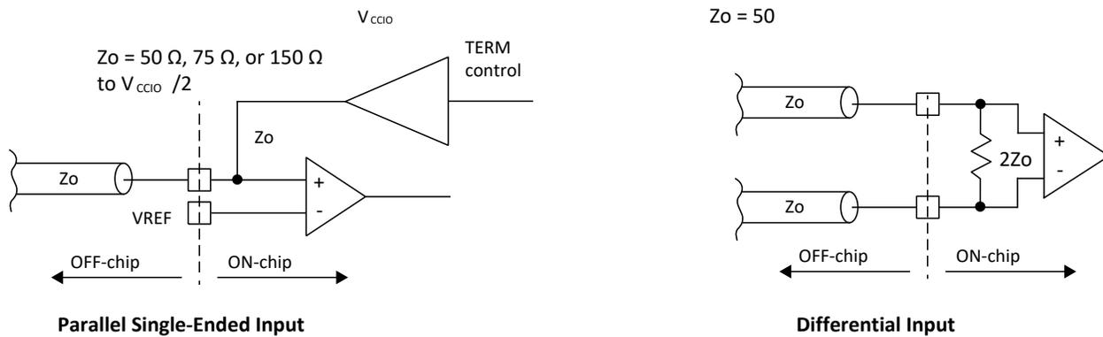
**Figure 3.1. On-Chip Termination**
