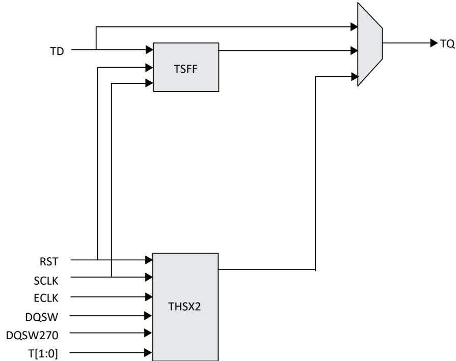
**Figure 2.24. Tristate Register Block on Bottom Side**
