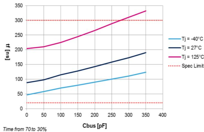
**Figure 14. Slave SDA rising time vs CBus Rup = 1.8 k $\Omega$ ,  $V_{DD}$  = 5 V,  $-40 < T_J < 125$  °C**
