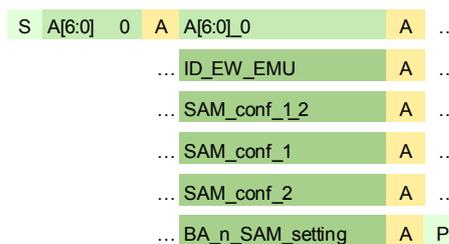
**Figure 39. Emulate OTP bit with parity detection**
