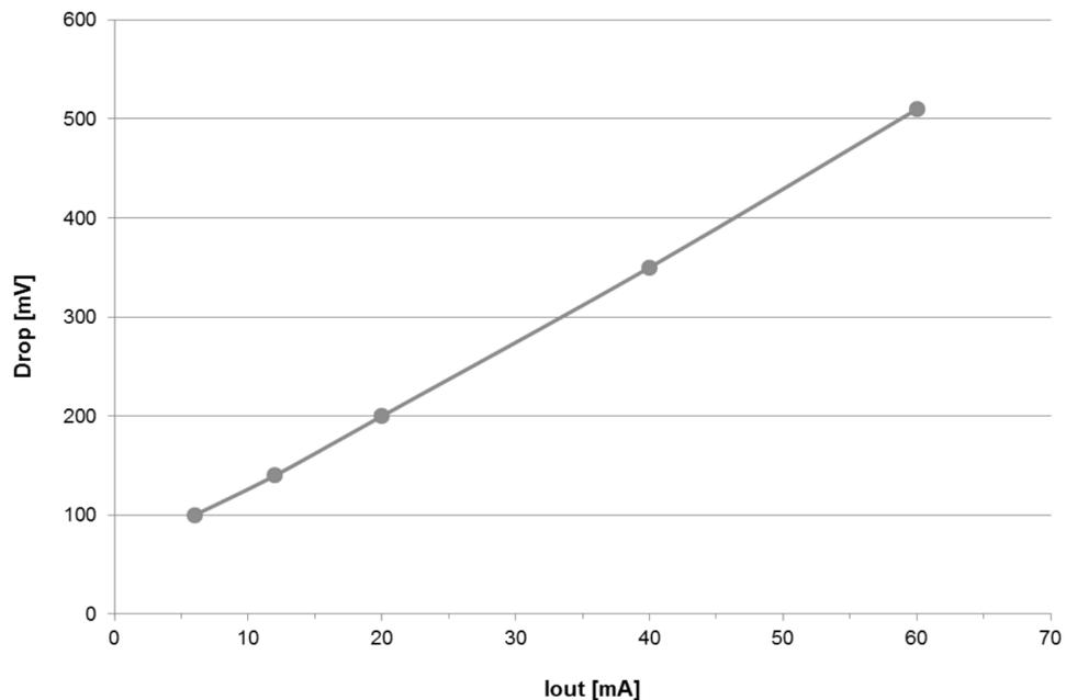
**Table 6. Minimum dropout voltage for certain current values ( $T_j = 25\text{ }^\circ\text{C}$ ; worst case simulated at target minus 3%)**
