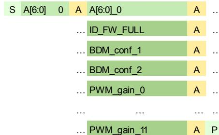
**Figure 25. With parity detection (32 bytes)**
