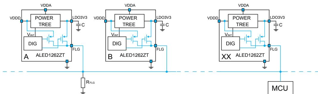
In case of dimming functions and FLG pin at high logic level due to one output in open condition (and/or thermal shutdown and/or  $R_{EXT}$  short), FLG behavior is different according to running dimming mode:
