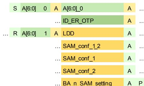
**Figure 43. Read back OTP bit with parity detection**
