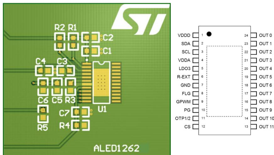
As already mentioned, to improve external conducted disturbance immunity, a serial resistor can be added to analog power supply pin ( $V_{DDA}$ ) before C3 and C4 to constitute a low-pass filter, and a serial resistor on digital power supply pin ( $V_{DDD}$ ) after C1 and C2 to avoid internal resonant effects (EMI conducted immunity section). These resistors are not placed on the following PCB example.
