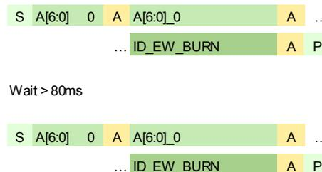
**Figure 41. Burn OTP bit with parity detection**
