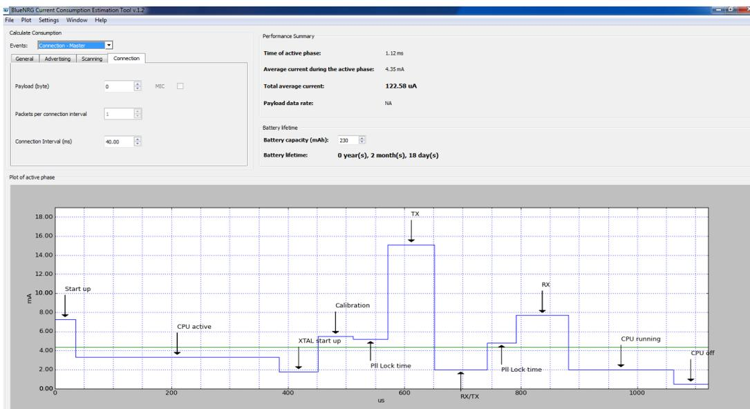
**Figure 6. Typical current consumption profile at 0 dBm**
