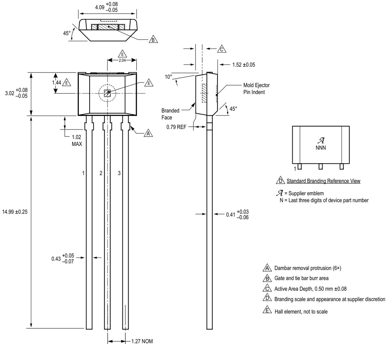
Figure 6: Package UA, 3-Pin SIP, Matrix Style
