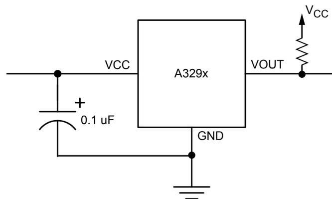
**Figure 4: Typical Basic Application Circuit**
