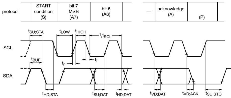
Rise and fall times refer to  $V_{IL}$  and  $V_{IH}$
