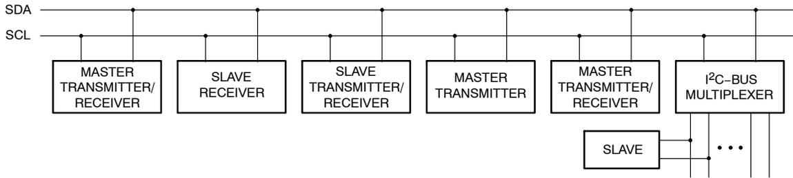
Figure 16. System Configuration
