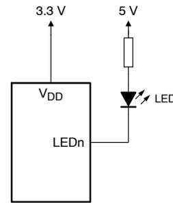
**Figure 13. Device Supplied by a Lower Voltage**
