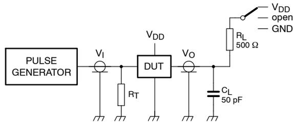
$R_L$  = load resistor.
