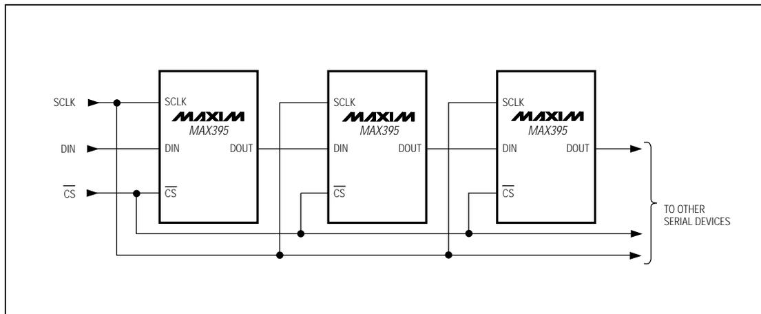
Figure 5. Daisy-Chained Connection
