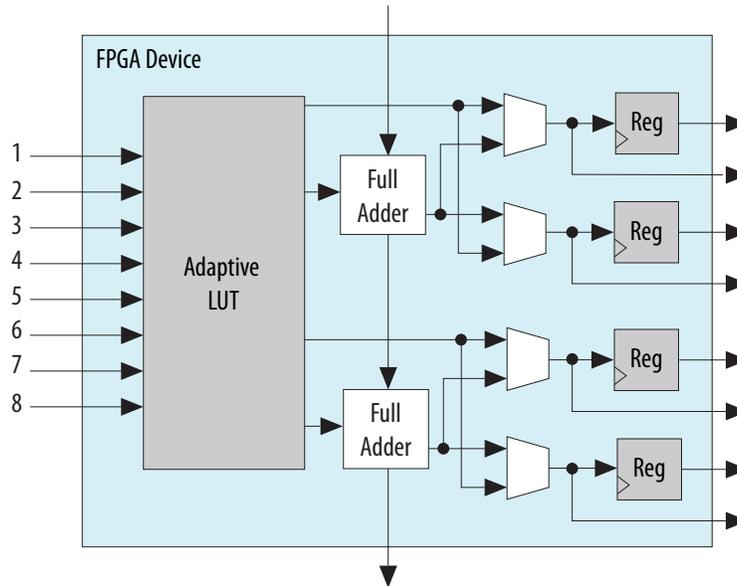
The Intel Quartus Prime Pro Edition software optimizes your design according to the ALM logic structure and automatically maps legacy designs into the Intel Cyclone 10 GX ALM architecture.
